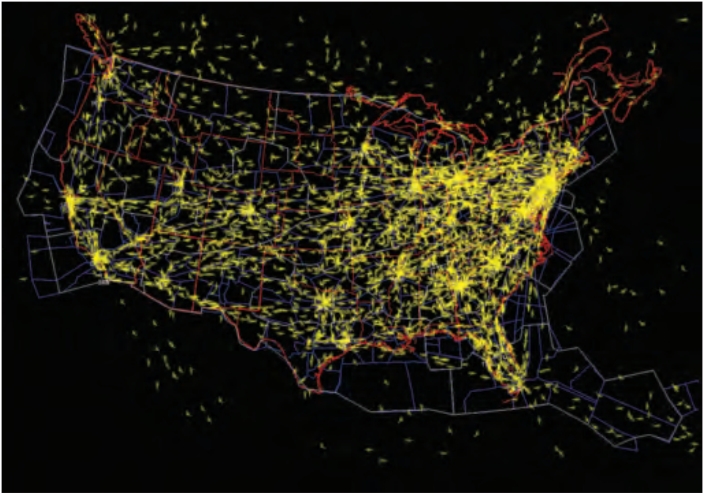
Future air traffic management concepts evaluation tool (FACET) uses live air traffic feeds and real-time weather information to process thousands of aircraft trajectories across the U.S. Air dispatchers use FACET to select more efficient routes based on capacity and weather conditions.
