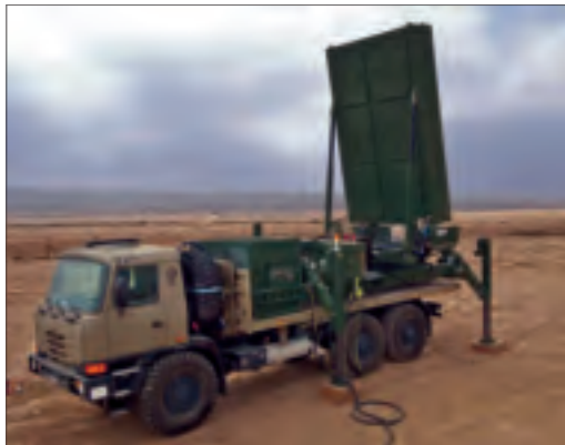
The EL/M-2084 provides very accurate target location information throughout the targeted rockets' trajectories, enabling the interceptor-missile to be directed accurately toward its target.
