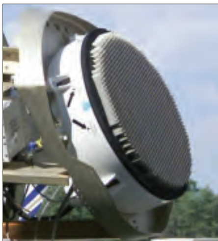
The AN/APG-81 AESA will provide near-simultaneous air-to-ground and air-to-air radar modes for the Joint Strike Fighter.
