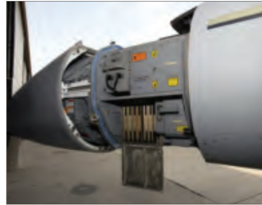
The APG-79 AESA was developed for the Navy F/A-18E/F.
