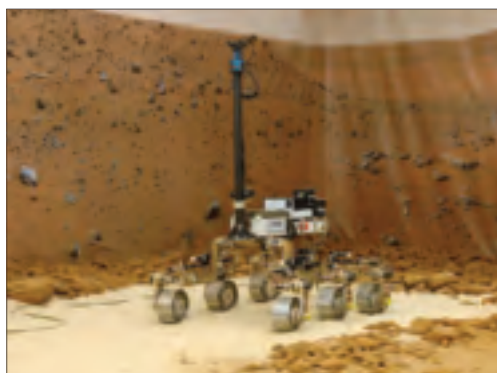
Astrium’s Locomotion Performance Model, Bruno, sits in the Astrium Mars Yard. Credit: EADS-Astrium.
