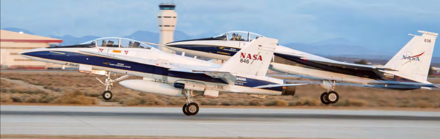
Photographing shockwaves: A NASA F/A-18B, left, carries a camera pod on its way to photograph an F-15B, right, that will soon be flying supersonically.
