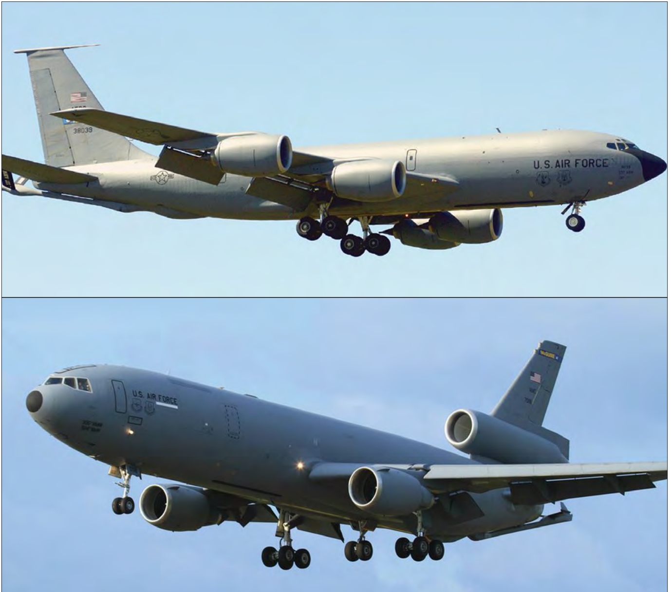
The KC-46A tanker will be about 20 percent larger than the KC-135 top, and about 20 percent smaller than the KC-10.
