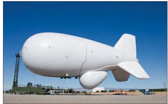
A Joint Land Attack Cruise Missile Defense Elevated Netted Sensor System, or JLENS. Plans to fly the radar-equipped aerostats near Washington, D.C., are uncertain.
