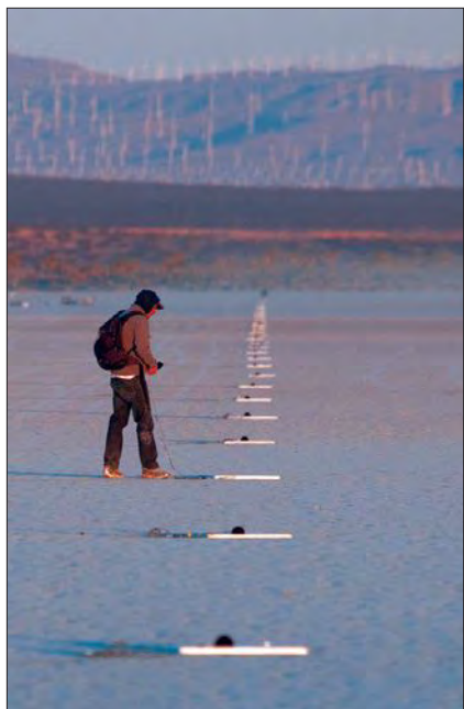
Rumble in the desert: A researcher adjusts a microphone to record the short-lived "evanescent" shock waves that sometimes reach the ground when planes fly supersonically.
