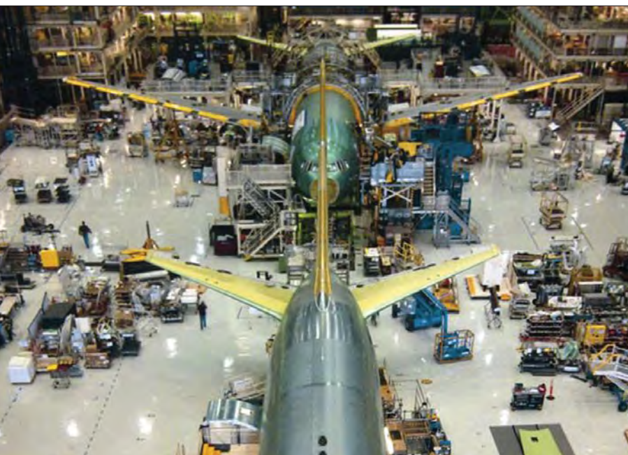
Efficiency drive: Boeing will build the KC-46A tanker on the 767 production line at Everett, Wash.
