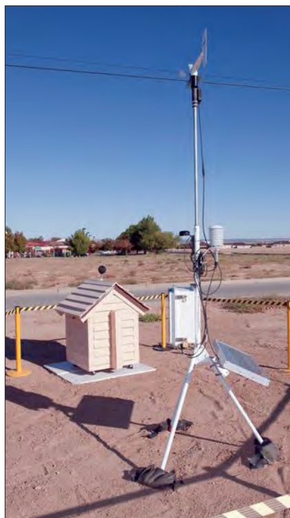
Ground truth: Sonic boom recorders gathered data while residents at Edwards Air Force Base, Calif., noted reactions to the booms. The doghouse contains SNOOPI, short for Supersonic Notification of OverPressure Instrumentation.
