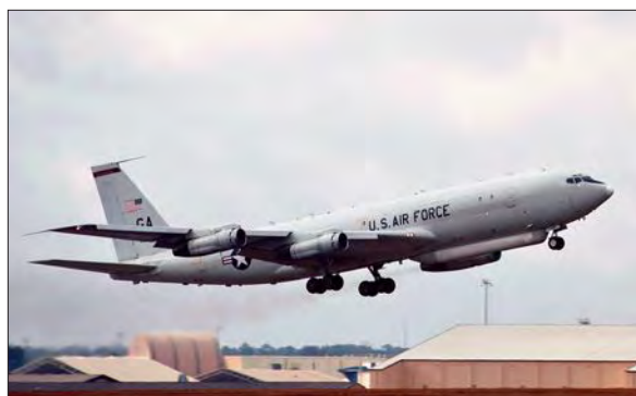
A canoe fairing protects the radar carried by an E-8C Joint Surveillance Target Attack Radar System plane. Radars could challenge video cameras for roles in targeting and surveillance.
