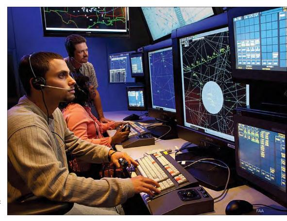
Air traffic controllers track flights on the En Route Automation Modernization system. Upgrades to ERAM will allow controllers at each of the nation's 20 air traffic control centers to track as many as 1,900 aircraft at once.
