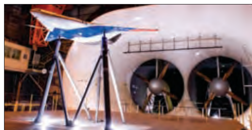
The X-48C completed a 300-hr test in the 30x60 wind tunnel facility at NASA Langley. (Photo by Bob Ferguson, Boeing.)
