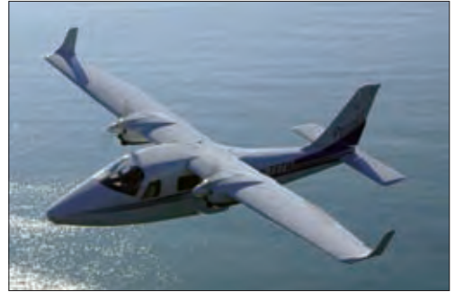
Tecnam this year introduced to the U.S. market the P2006T light twin with economical 100-hp Rotax engines.
