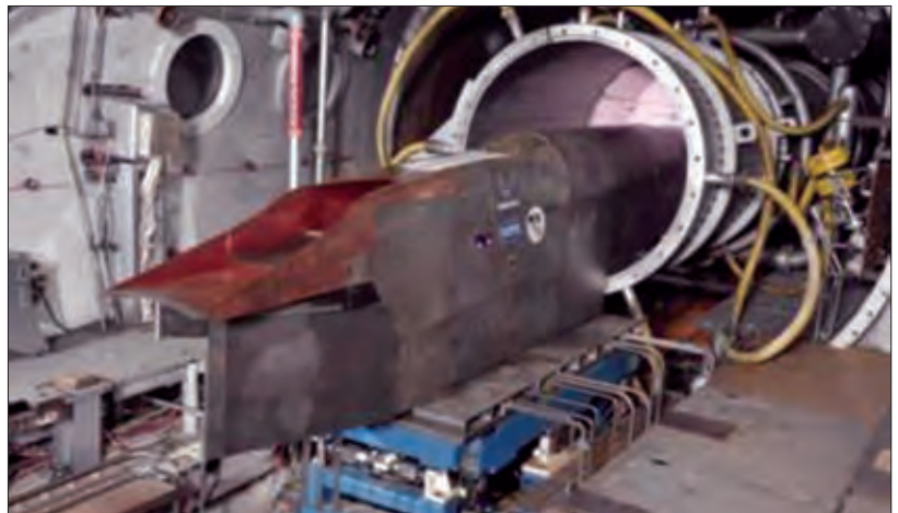
The first-ever scramjet propulsion test at AEDC took place when the DARPA FaCET was tested in the center's Aerodynamic and Propulsion Test Unit. (USAF photo.)
