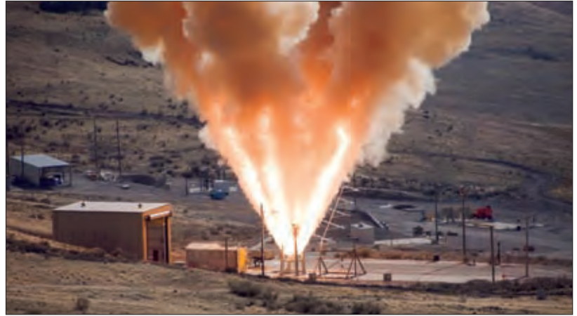
NASA and ATK successfully test an Orion launch abort system motor in a 5.5-sec test in the Utah desert at Promontory.
