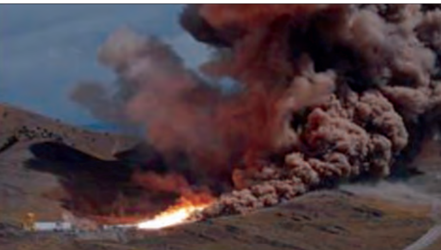
The Ares I first stage motor undergoes test firing in Utah.
