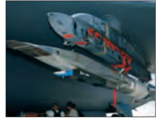
The X-51A stack is mated to a B-52H with a JDAM interface.
