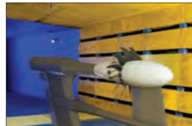
In September, a one-fifth-scale open-rotor propulsion rig began a new test campaign in the NASA Glenn anechoic 9x15-ft wind tunnel.
