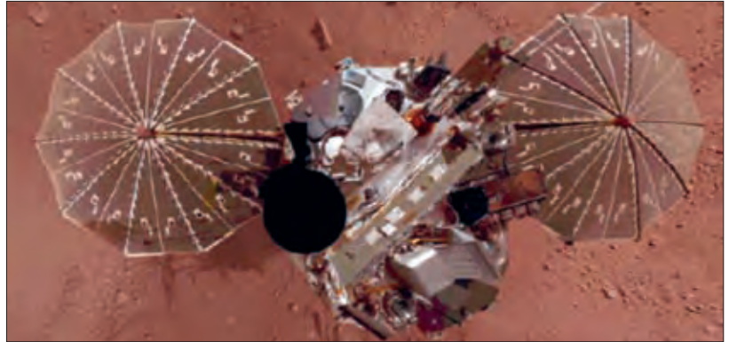
The Mars Phoenix Lander uses ATK's UltraFlex solar array wings.
