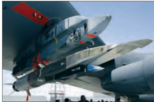
The X-51A SED-WR is poised to demonstrate the first-ever sustained flight beyond Mach 6 of a hydrocarbon-fueled and -cooled air-breathing engine.
