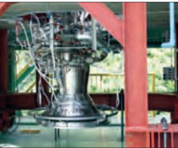
In Japan, the LE-8 LOX/natural gas rocket demonstrated its flight feasibility in tests this summer.
