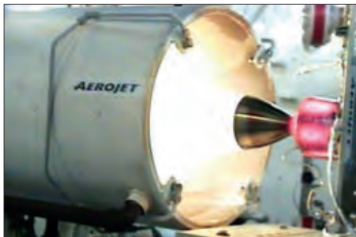
The MR-80 Ares roll control engine undergoes testing at Aerojet.
