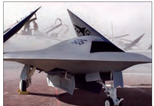
The fighter-sized Navy X-47B UCAV can conduct long-range, high-endurance missions including ISR and precision strikes.
