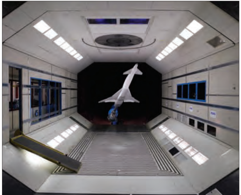
In Europe, a study of an environmentally friendly high-speed aircraft featured low-speed wind tunnel testing.
