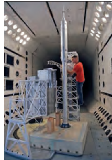
An engineer inspects part of the simulated launch tower between scale model tests of NASA's Ares I-X rocket in the Langley transonic dynamics tunnel.
