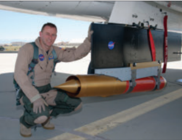
NASA research pilot Jim Less checks out the CCIE experimental jet engine inlet mounted underneath NASA's F-15B prior to a test flight. Photo courtesy NASA/Tony Landis.
