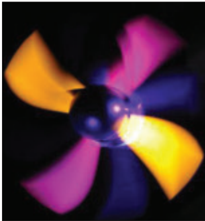
A rotating propeller is coated with pressure (magenta) and temperature (yellow) paints. Obtained by DLR and the University of Hohenheim.
