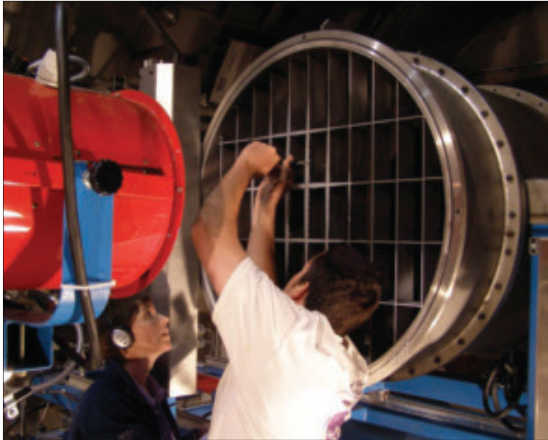
NASA engineers measure ice accretion thickness on a cloud uniformity grid during a PSL-3 system checkout.
