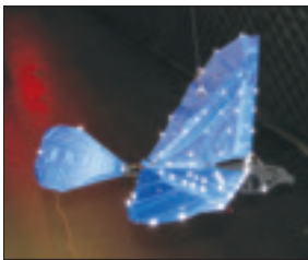
The University of Maryland conducted a flight test of a custom-built avian-scale flapping wing.
