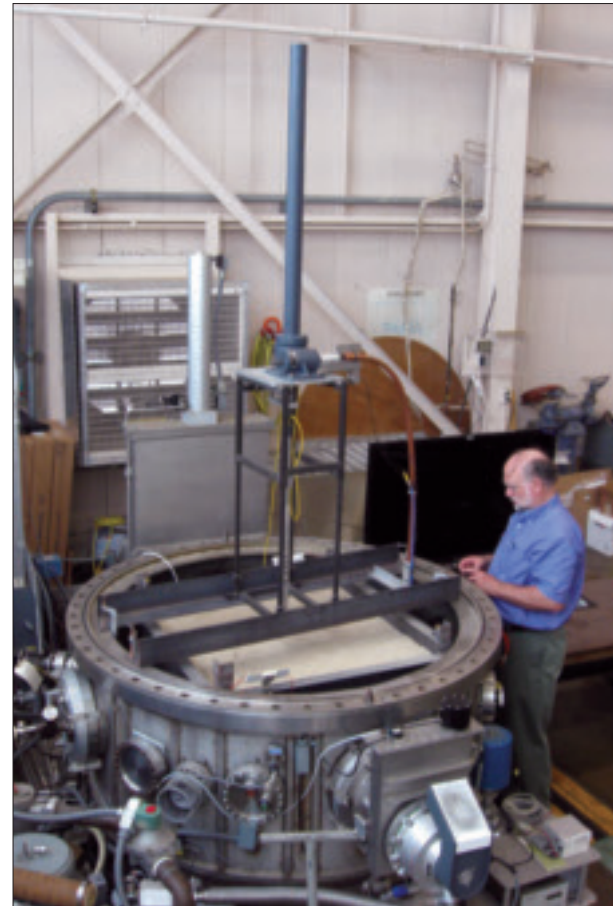
In the large vacuum chamber dedicated to tests involving large amounts of regolith simulant at NASA Glenn the soil bin rests in the lower, fixed base of the chamber.
