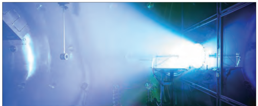
The VASIMR VX-200 engine can be propelled by chemicals such as argon, oxygen, and nitrogen. Credit: Ad Astra Rocket.
