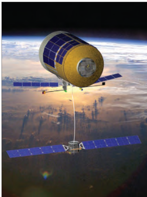
In the PROPEL-Tug concept, Japan's H-2 Transfer Vehicle and a multiton payload could be used to demonstrate electrodynamic tether propulsion. Credit: Tethers Unlimited.
