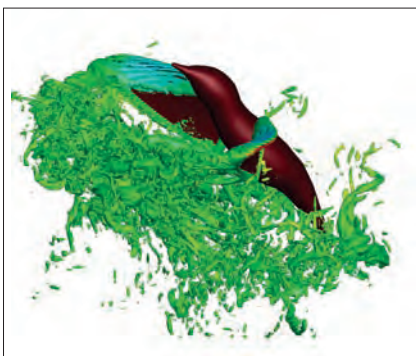
Images of the flow around a hummingbird in hovering flight show downstroke and upstroke. The color indicates pressure in the flow. Credit: Haoxiang Luo and Tyson Hedrick.
