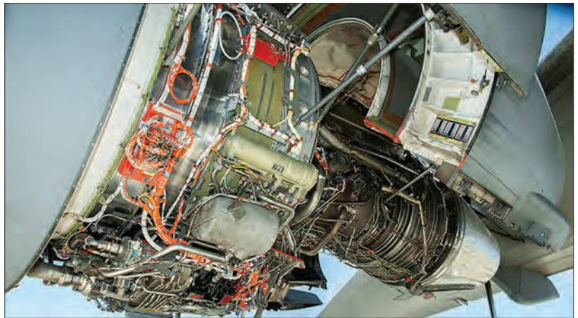
Researchers demonstrated online wire chafing fault detection on C-17 engines at NASA Dryden. Credit: Ken Ulbrich, NASA Dryden.
