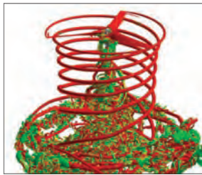
A tiltrotor aeroacoustic model wake features different levels of Richardson extrapolation error control.
