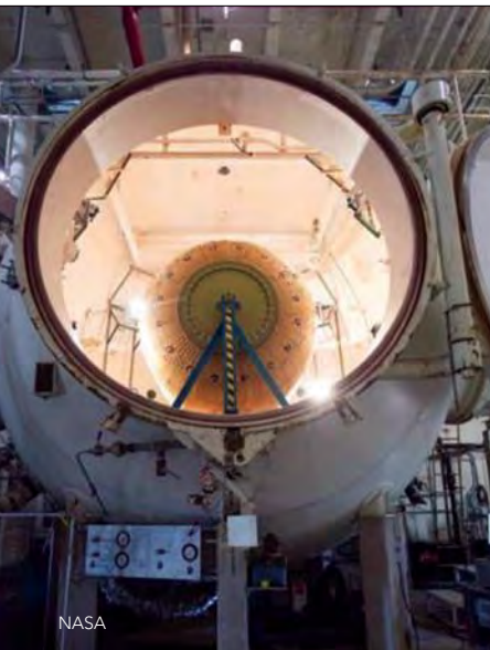
An inflatable pressure vessel undergoes a creep burst test at NASA's Johnson Space Center to determine material properties, including failure pressures and creep times.
