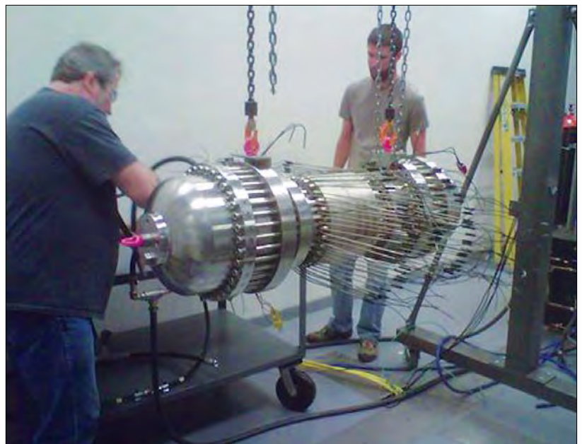
Sunpower's 12 kilowatts-electric power conversion unit with electrically heated heater head.
