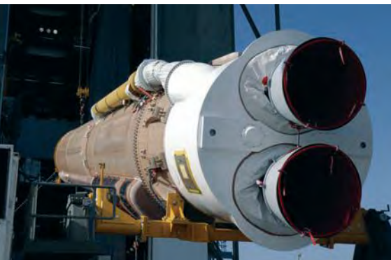
An Atlas 5 with RD-180 rocket engines built by the Russian company NPO Energomash.
