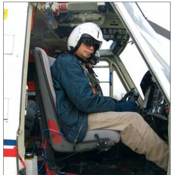
An instrumented Bell 412 helicopter provided insights into the effects of whole-body vibration on aircrews under research conducted by the National Research Council of Canada.
