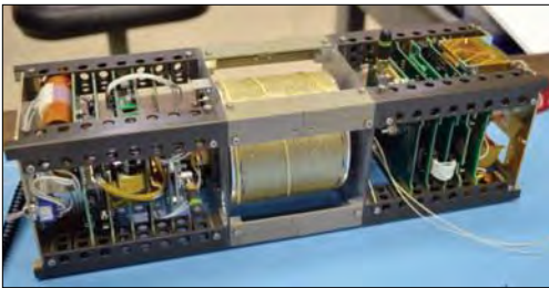
The Naval Research Laboratory's TEPCE 3U CubeSat.
