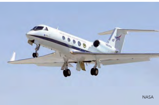
A modified Gulfstream 3 is NASA's testbed for flexible-wing-flap research.
