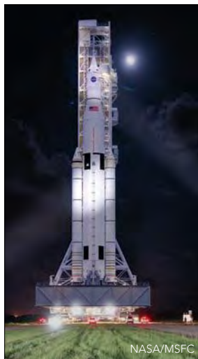
Artist concept of NASA's Space Launch System. Marshall Space Flight Center developed an operational modal analysis process for the SLS rollout using a finite element model of the vehicle-launcher assembly.
