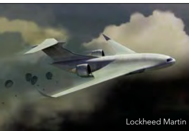
Lockheed Martin's hybrid-wing-body concept airlifter is designed to burn 70 percent less fuel than the C-17.
