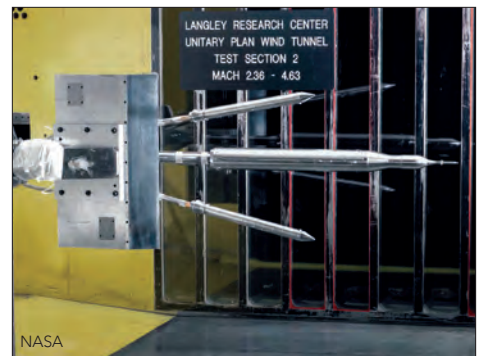
NASA's Space Launch System is undergoing wind-tunnel tests, including at the Langley Unitary Plan Supersonic Wind Tunnel in Virginia.
