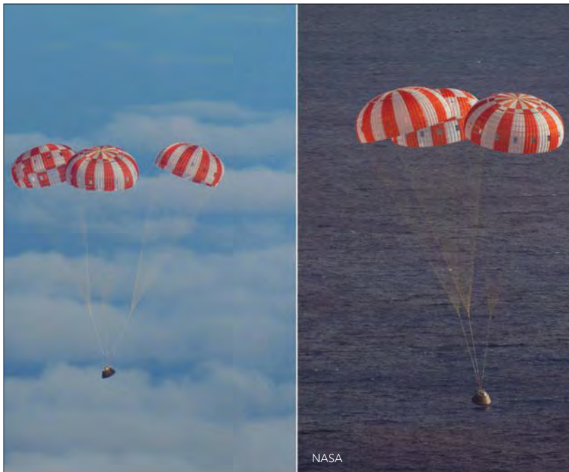
Three main parachutes of NASA's Orion spacecraft helped it descend to Earth after its December 2014 flight test. Since then, Orion has been undergoing detailed post-processing and data analysis.
