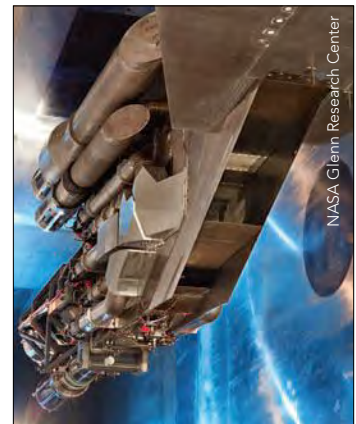
Phase 3 tests began in April in the 10'x10' Supersonic Wind Tunnel for the NASA/Air Force Research Laboratory's combined-cycle engine — large scale inlet for mode transition experiment.
