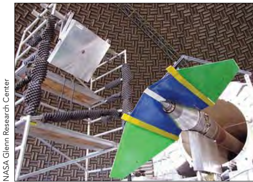
A scale model of an aft deck and tail of future supersonic airliner undergoes acoustic tests for exhaust noise at NASA's Glenn Research Center.
