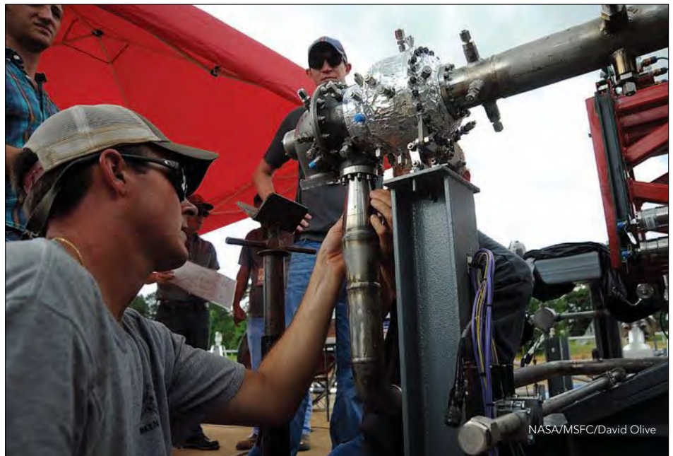
NASA engineers prepare a 3D-printed turbopump for a test at NASA's Marshall Space Flight Center in Alabama.
