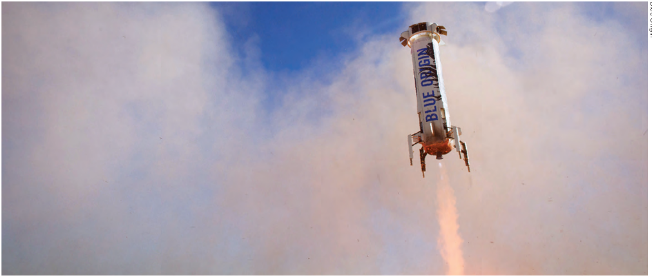
▲ Blue Origin's New Shepard booster executes a controlled vertical landing.
