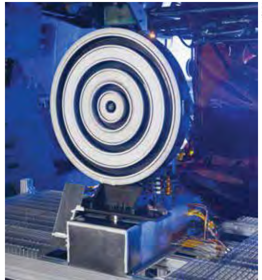
▲ The X3 Nested Hall Thruster is mounted to a specially made thrust stand at NASA's Glenn Research Center. It was tested to a power level of 100 kW.
