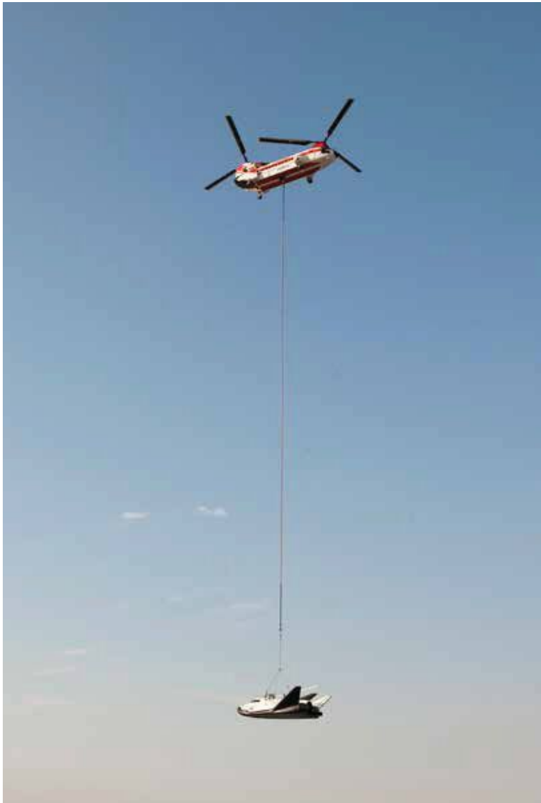
◀ Sierra Nevada's Dream Chaser is lifted off a ramp at NASA Armstrong by a Chinook helicopter for a captive carry flight.
