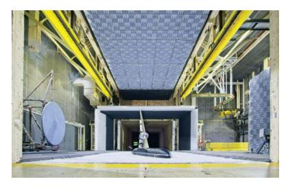
▲ Researchers test the highlift variant of the Common Research Model in the 14-by-22-foot (4.3-by-6.7meter) subsonic wind tunnel at NASA's Langley Research Center in Virginia to substantiate that a slat-gapfiller design can effectively reduce the noise signature from the airframe.
