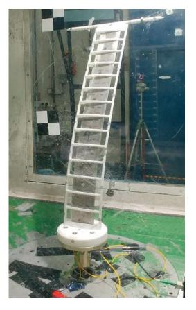
The Pazy wing is shown in its highly deformed state in the Technion wind tunnel at a 7-degree angle of attack and a 55-meters-per-second free stream.
