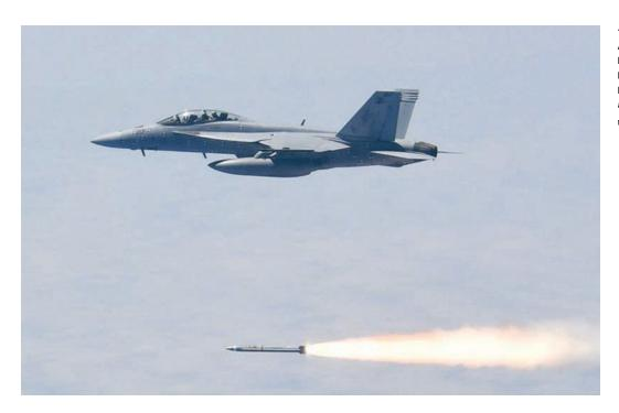
◆ The AGM-88G Advanced Anti-Radiation Guided Missile Extended Range missile was launched from a U.S. Navy F/A-18 Hornet aircraft during a live-fire test this year.
