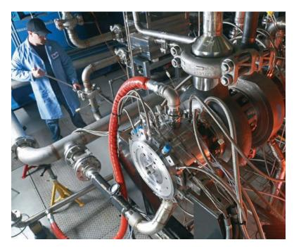
▲ Supercritical carbon dioxide power generation systems consist of compact, more efficient components. The desk-sized 10-megawatt-electric supercritical carbon dioxide turbine designed by General Electric and Southwest Research Institute yields the highest power density of any industrial turbine at higher efficiency, according to Southwest Research Institute.
