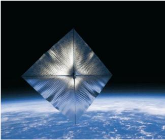
▲ Renderings of NASA's prototype 80-meter-squared Advanced Composite Solar Sail System show it as it would look in the process of unfurling (left) and then complete.
