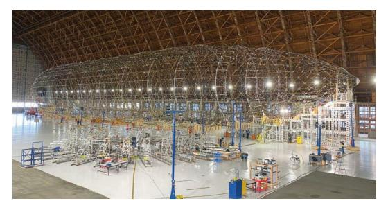
This photo of the completed internal airframe of the Pathfinder 1 airship was released in October by LTA Research, owned by Google billionaire Sergey Brin. The vehicle, in construction at Moffett Field in California, will measure 123 meters by 20 meters. LTA Research
