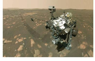
NASA's Perseverance rover generated a photo of itself and the Ingenuity Mars Helicopter this year with its Wide-Angle Topographic Sensor for Operations and Engineering, or WATSON, camera.
