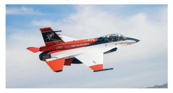
The U.S. Air Force Test Pilot School's Ione X-62A Variable In-flight Simulator Test Aircraft, or VISTA, has been upgraded to include multiple data links for command and control and
