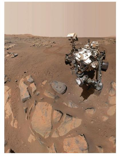
NASA's Perseverance rover generated this selfie on Mars in September over a rock nicknamed Rochette. The rover's robotic arm drilled two holes in the rock to extract core samples.
