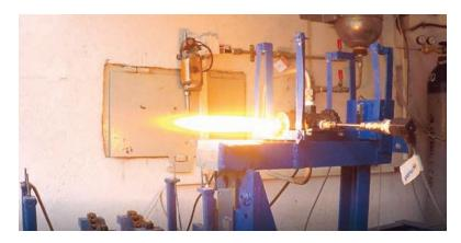
A demonstration of a wateraugmented hybrid ducted rocket showed that adding a secondary stream of water can increase the thrust and specific impulse by as much as 70%. The static test was at the Fine Rocket Propulsion Center of the Technion-Israel Institute of Technology.
