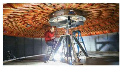
▲ NASA performed ground testing this year in preparation for the planned Low-Earth Orbit Flight Test of an Inflatable Decelerator in 2022.
