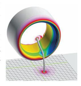
▶ The results of this computational fluid dynamics simulation show a ground vortex in an inlet in crossflow. The prediction of the existence of the vortex is notoriously sensitive in CFD to boundary conditions, crosswind and grid resolution. The results provide guidelines for setting up problems based on actual test data.
