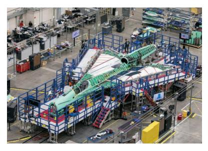
▲ This year workers joined the wing, tail assembly and fuselage of the Quiet SuperSonic Technology, or QueST, aircraft at Lockheed Martin Skunk Works in California.
