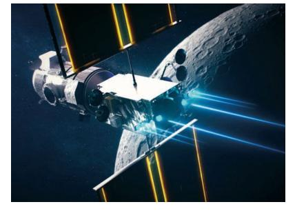
An illustration of the Gateway's Habitation and Logistics Outpost and Power and Propulsion Element modules.
