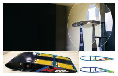
▲ This morphing wing can change shape during flight by selecting one of its two configurations. At top, the wing is instrumented and prepared for wind tunnel testing. At bottom left, the red and blue bistable device determines how stiff the wing is; additional actuators are on the upper airfoil surface. At bottom right, simulations predict the available morphed configurations.
