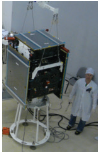
Prisma is mounted on the adapter and final electrical tests are performed. Image courtesy of SSC.
