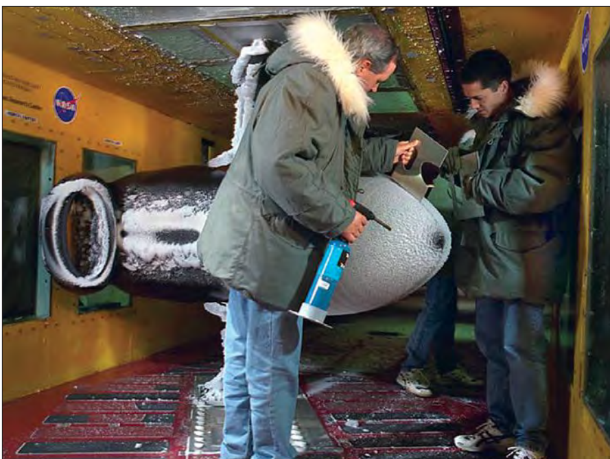
NASA researchers use a laser scanner to collect a 3D model of ice accretion. Credit: NASA
