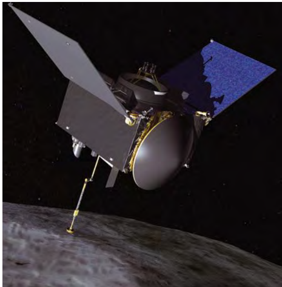
OSIRIS-REx, shown in an artist's rendering, will extend an arm to collect up to 2 kilograms of regolith from the near-Earth asteroid Bennu and return the sample to Earth.
