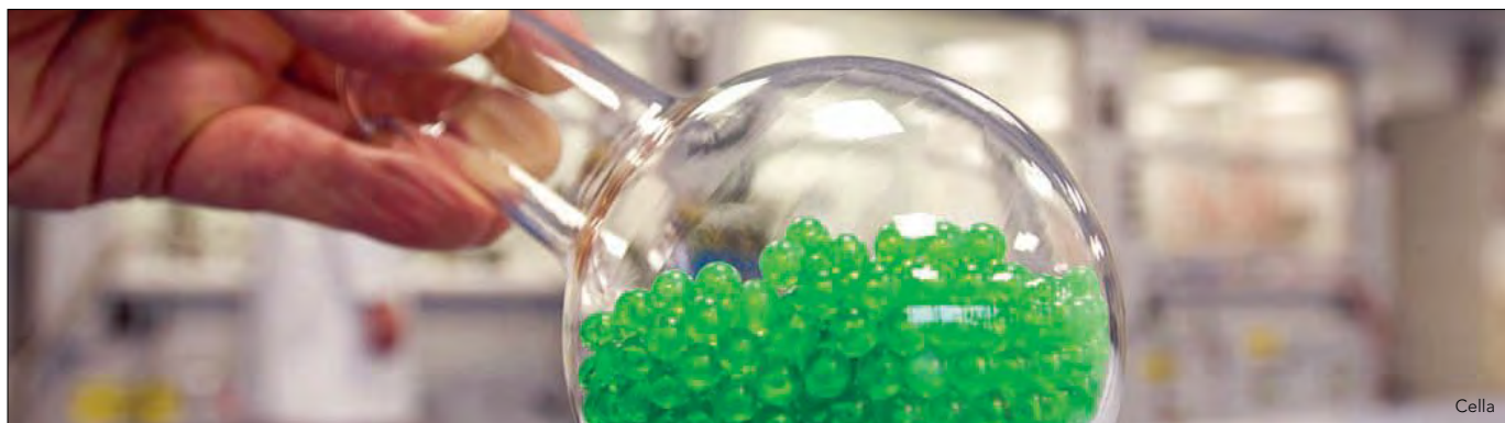
Each gram of flowable hydrogen pellets from Cella Energy of London can produce as much as a liter of hydrogen gas. Cella expects to sign a contract with a subsidiary of Safran to develop solid hydrogen to supply electric power to airliners.
