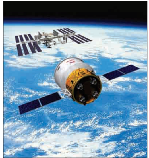
The Cygnus advanced maneuvering spacecraft is Orbital Sciences' cargo delivery vehicle. Cygnus will perform ISS resupply flights under NASA's commercial resupply service contract.
