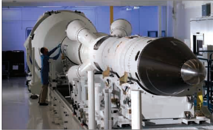
Last September the Orion launch abort system underwent ground vibration tests at Orbital Sciences’ facility in Dulles, Va. The 53-ft-long assembly was an inert test article; a live pad-abort test of the system will be conducted this spring at White Sands.
