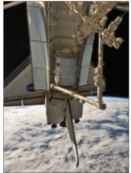
Canadarm2 grapples the Leonardo MPLM from Discovery's payload bay for relocation to a port on the Harmony node of the ISS.
