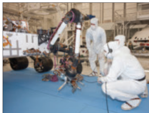
Curiosity’s 7.5-ft robotic arm, which will use a percussion device to break rock into powder, is much stronger than the 3-ft MER arms.
