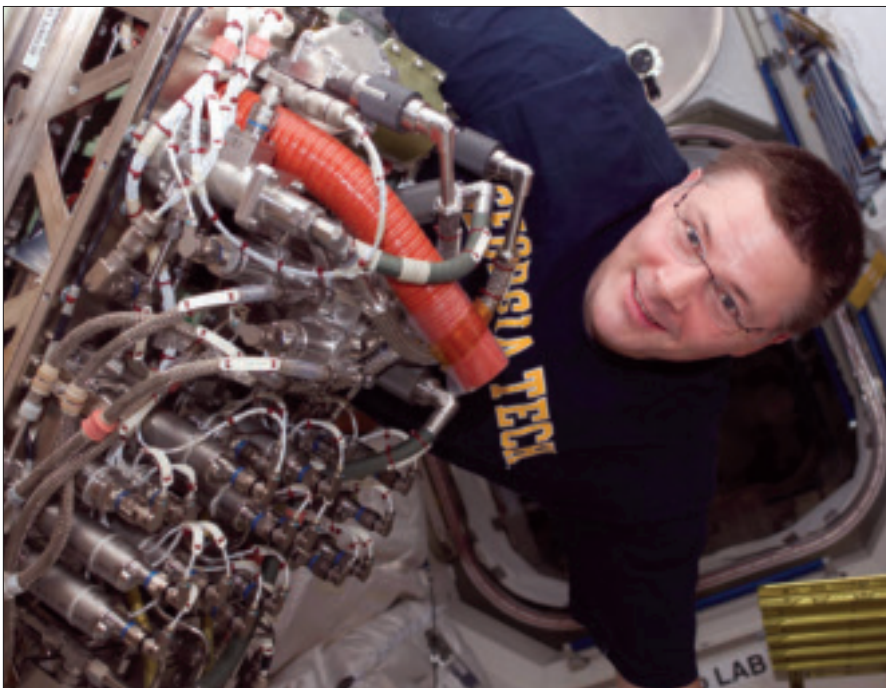
In the Tranquility node, NASA astronaut Doug Wheelock, Expedition 25 commander, works to install the new Sabatier system that will extract more water out of the ISS atmosphere.
