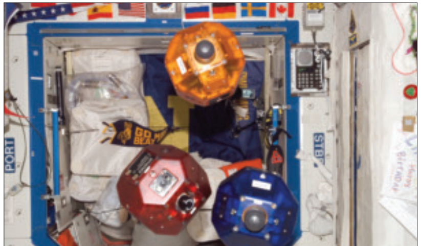
SPHERES, stowed inside the Destiny lab, were designed to test control algorithms for spacecraft by performing autonomous rendezvous and docking maneuvers inside the station. Their progressively more complex two- and three-body maneuvers include docking—to fixed, moving, and tumbling targets—as well as evaluating formation flying and prospective searching for lost satellites.
