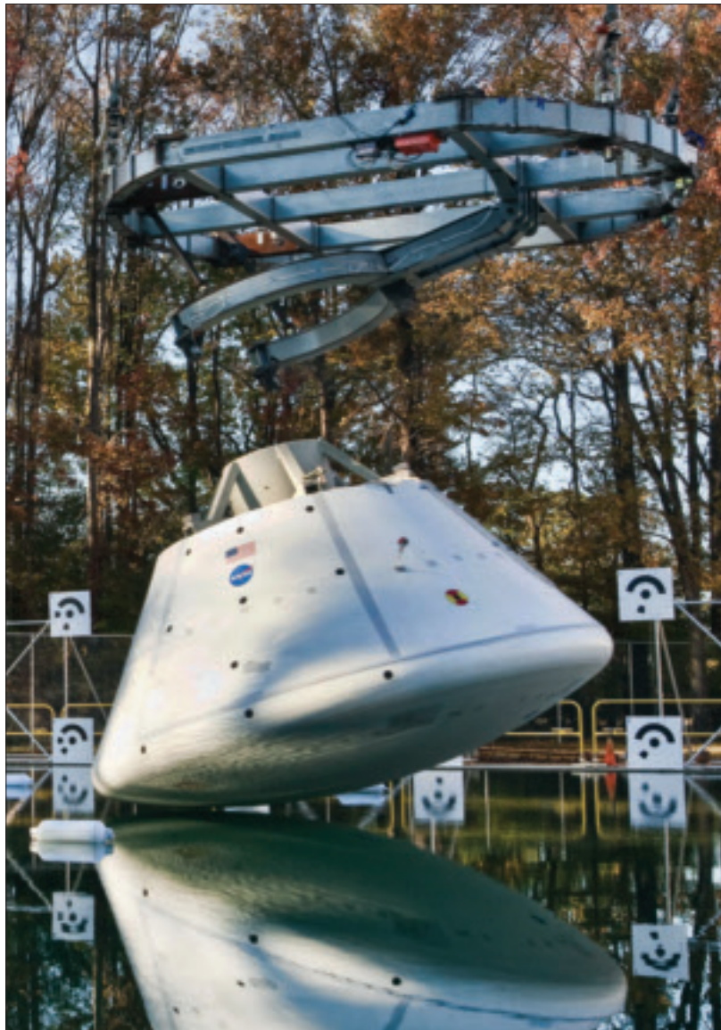
Engineers at NASA Langley conducted the third drop test of the Orion test article as part of Phase 1 water impact testing on November 8. The capsule was hoisted about 20 ft above the ground with a pitch of 17 deg. It reached a horizontal velocity of about 22 mph before splashing into the Hydro Impact Basin. Credit: NASA/Sean Smith.
