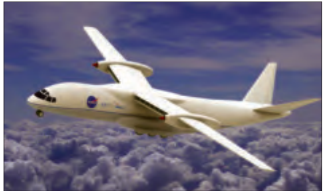
The turboelectric distributed propulsion concept proposed in the N3-X study could also be used to power a more conventional tube-and-wing aircraft configuration, according to the NASA Glenn engineers who are conducting the research.
