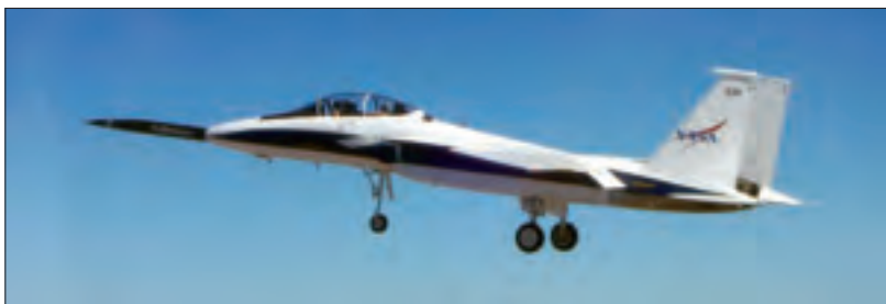
NASA's F-15B testbed aircraft flew in the first evaluation flight of the joint NASA/Gulfstream Quiet Spike project, which seeks to verify the structural integrity of the multisegmented, articulating spike attachment designed to reduce and control a sonic boom. Credit: Lori Losey.
