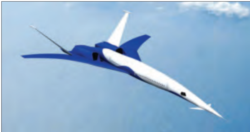
Icon II is Boeing’s concept for an N+3 SST configuration. Boeing research concluded that N+2 SST concepts are unlikely to meet fuel efficiency and sonic boom mitigation goals at the same time, so they identified a preferred N+3 concept that shows the potential to meet or exceed nearly all the NASA goals for N+3.
