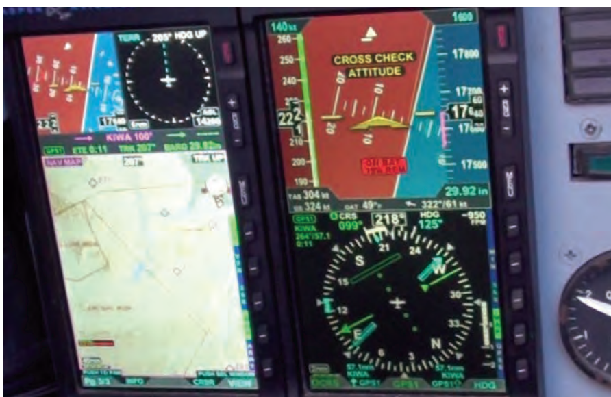
Recover or die: The cockpit display of an A-4 training jet shows its wings nearly perpendicular to the ground after a severe stall. Credit: Aviation Performance Solutions.
