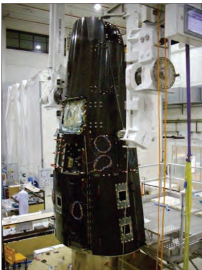
The front and rear segments mated into a single assembly. Credit: ESA/Thales Alenia Space.
