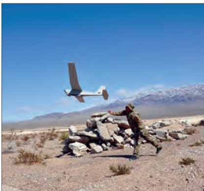
Used by U.S. military troops in Afghanistan, the 6-kilogram Puma has been approved by the FAA for flights in the Arctic. Credit: AeroVironment
