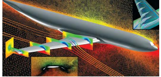
The intensive calculations needed to generate this CFD visualization — a mesh adaptation simulating a transport aircraft in a high-lift configuration — were performed by a NASA high-performance computer.
