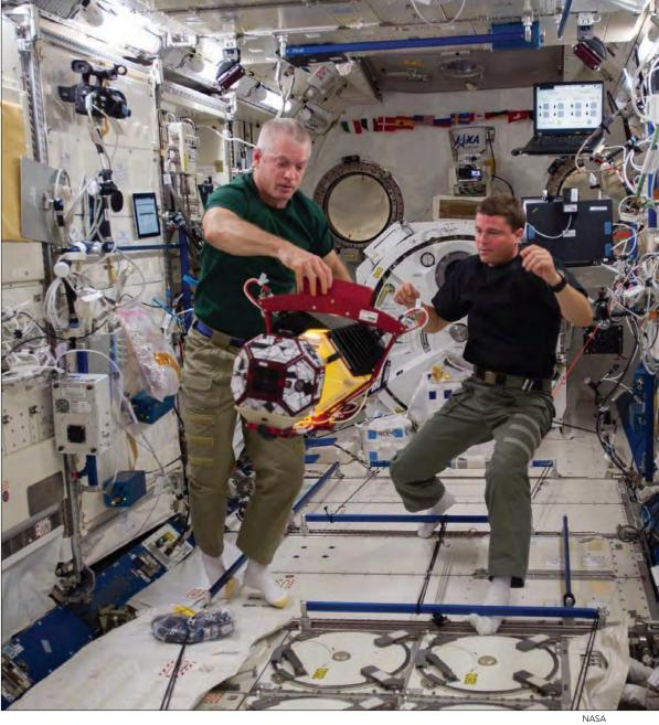
Steve Swanson, left, and Reid Wiseman conduct test runs of the SPHERES-Slosh experiment, which uses soccer-ball-sized Synchronized Position Hold, Engage, Reorient, Experimental Satellites to examine how liquids move inside containers in microgravity.
