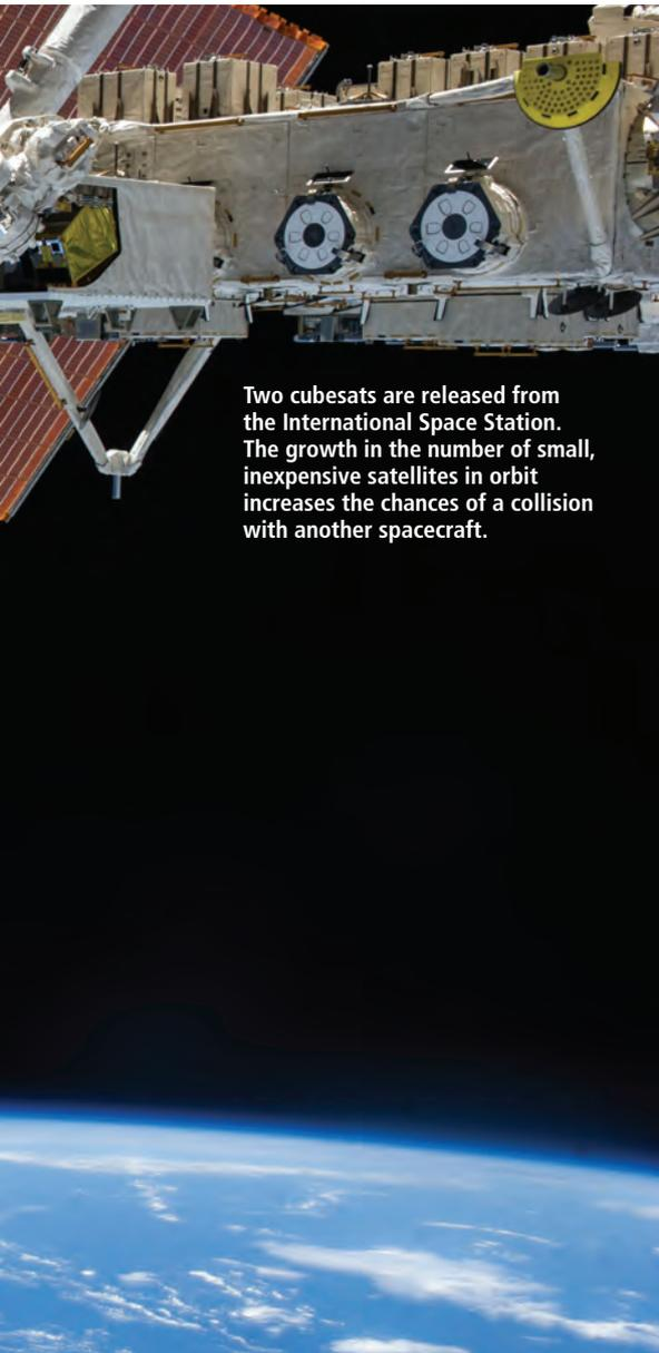
Two cubesats are released from the International Space Station. The growth in the number of small, inexpensive satellites in orbit increases the chances of a collision with another spacecraft.
