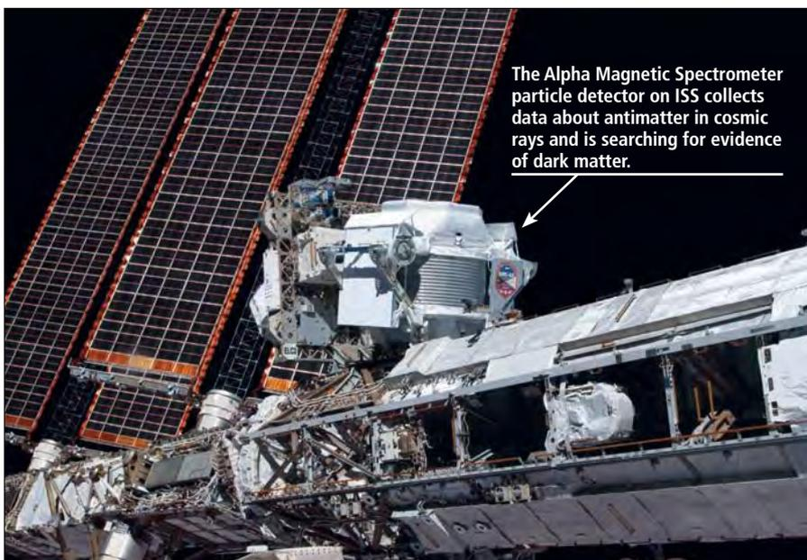
The Alpha Magnetic Spectrometer particle detector on ISS collects data about antimatter in cosmic rays and is searching for evidence of dark matter.
