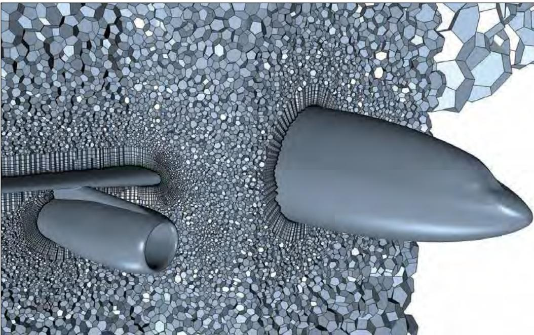
The rapid generation of 3-D meshes around aircraft models, a key step in the CFD process, will become even more important as more powerful computers enable higher-resolution simulations, according to a NASA report.
