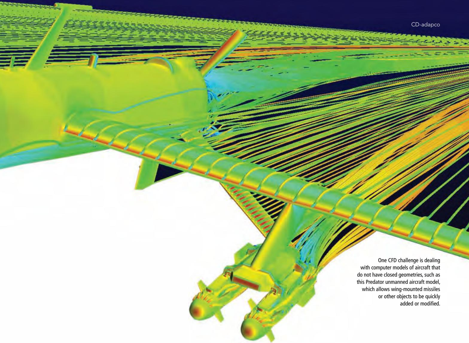
One CFD challenge is dealing with computer models of aircraft that do not have closed geometries, such as this Predator unmanned aircraft model, which allows wing-mounted missiles or other objects to be quickly added or modified.
