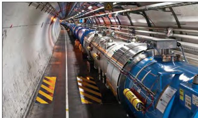
Superconducting electromagnets like those that guide particle beams in the Large Hadron Collider might someday protect astronauts from radiation by generating an intense magnetic field.
