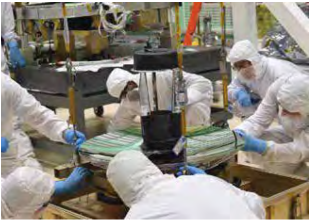
▲ Engineers and technicians check the fit of ICESat-2's telescope to its sling, before moving it into place on the instrument's optical bench.
