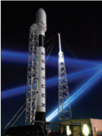
SpaceX's Falcon 9 booster stands on launch complex 40 at Cape Canaveral Air Force Station. Falcon 9's first stage generates more than a million pounds of thrust.
