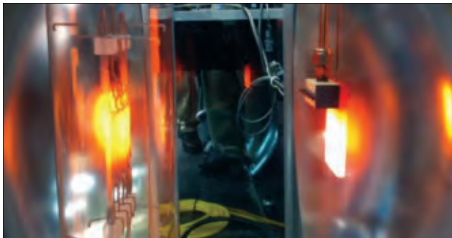
A segment of graphite is heated to 2,000 K by a 20-kW light during a February test at NASA Ames. Later tests will add channels and helium to simulate hydrogen propellant. Photo credit: David Murakami and Kevin Parkin.
