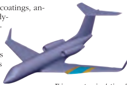
This computer simulation shows what the wing glove looks like and how it will be placed on the testbed aircraft. Image credit: NASA/Ethan Baumann.
