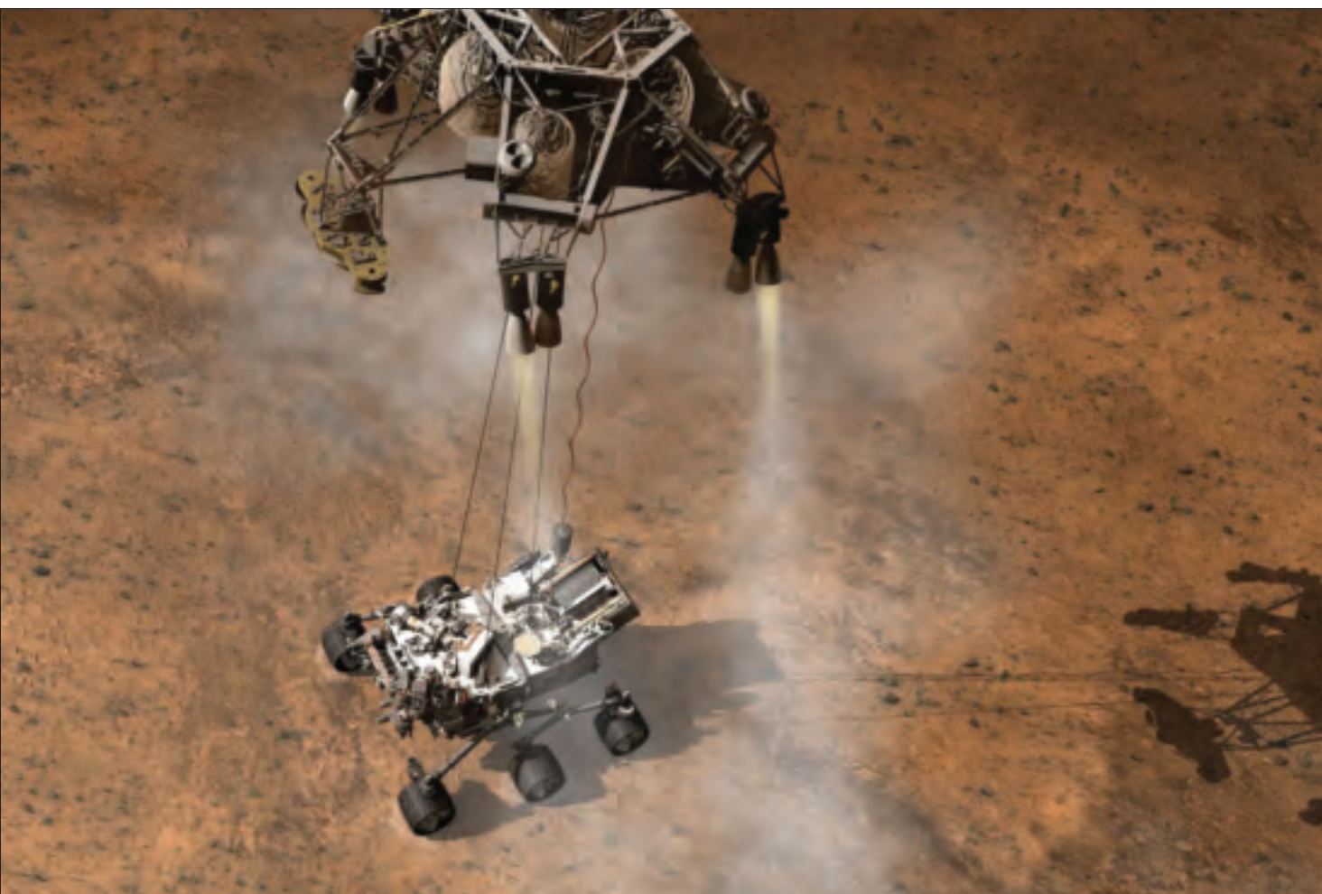
Curiosity touches down on the Martian surface. The MSL mission's EDL phase will begin when the spacecraft reaches the Martian atmosphere, about 81 mi. above the surface of the Gale Crater landing area, and ends with the rover safe on the surface of Mars. Credit: NASA/JPL-Caltech.
