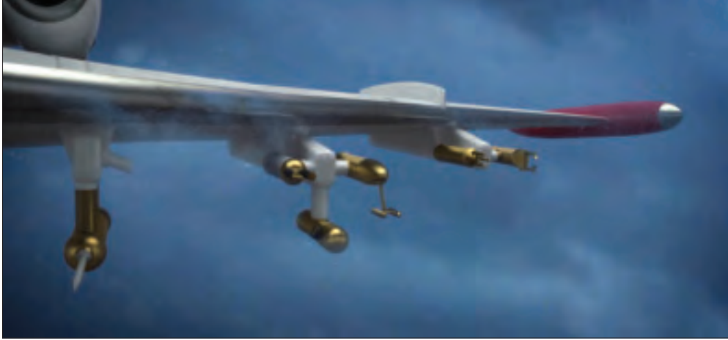
In 2013 NASA Glenn will fly a modified Gulfstream 2 research aircraft in the air over Darwin, Australia, an area known for ice storms with high levels of ice crystals. More than 20 meteorological instruments on the aircraft will collect data. Image credit: NASA/Eric Mindek.
