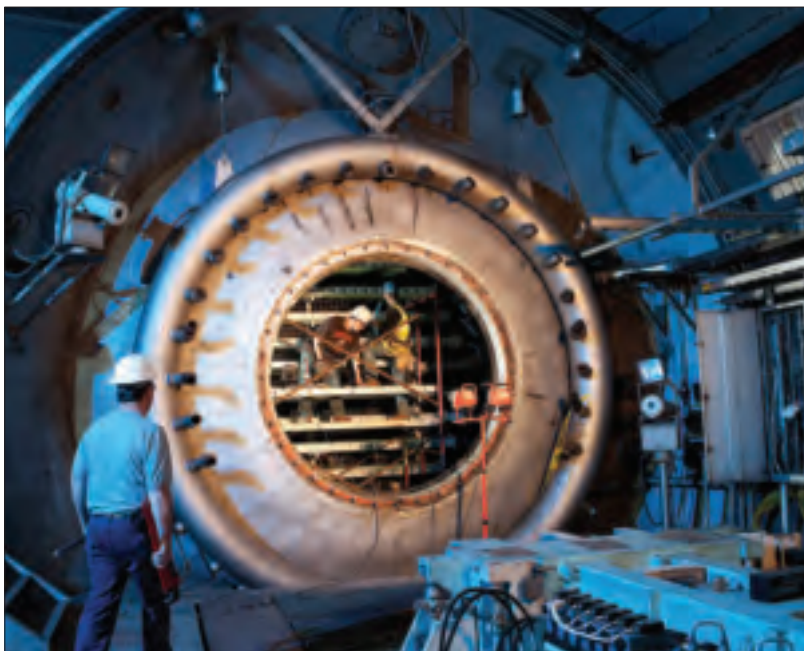
Water sprayers are installed in the jet engine icing test chamber at NASA Glenn. The sprayers will produce tiny ice crystals that can clog or damage engines.
