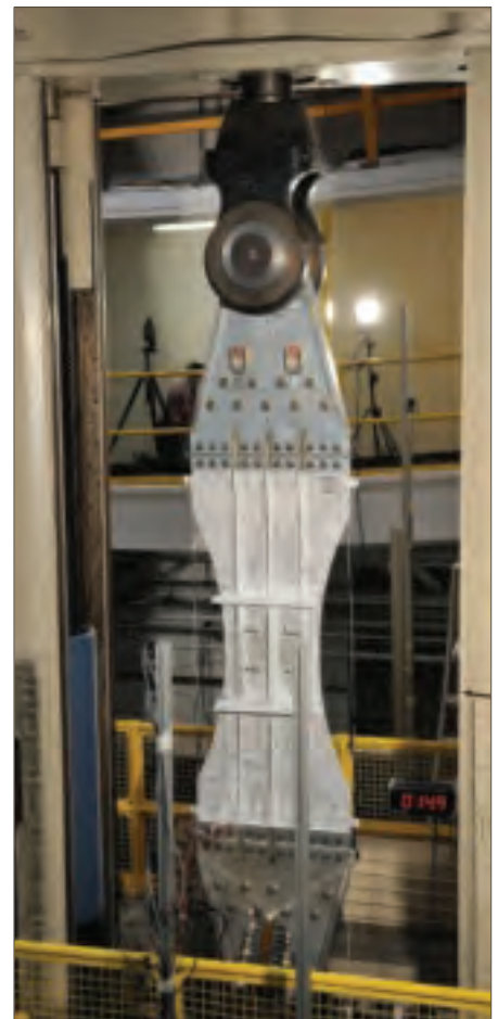
A PRSEUS tension panel with bolted repair is tested in the 1-million-lb machine at NASA Langley.
