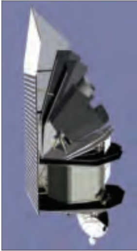
According to the B612 Foundation, "Sentinel is a space-based infrared survey mission to discover and catalog 90% of the asteroids larger than 140 m in Earth's region of the solar system." Credit: Ball Aerospace.
