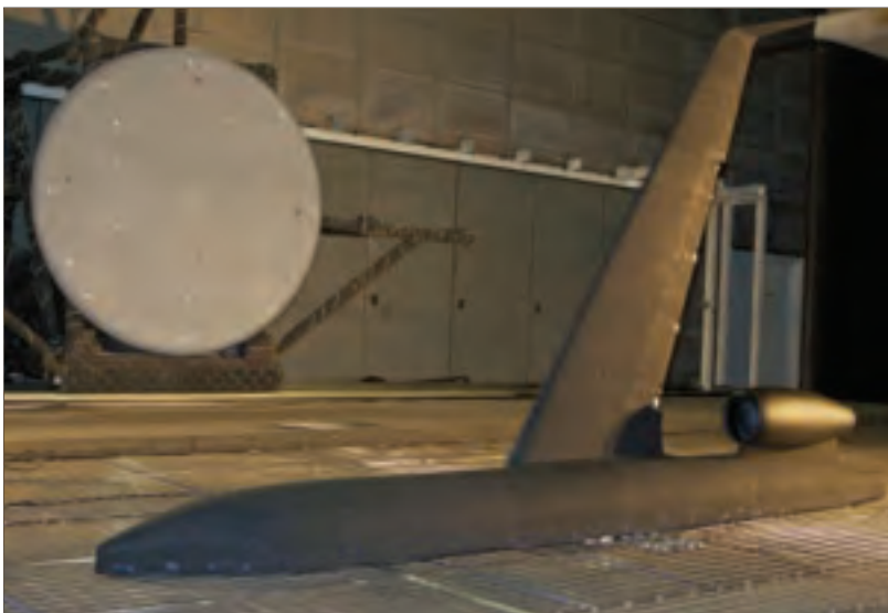
A semispan jet model has just completed testing in NASA Langley's 14x22 ft subsonic wind tunnel to evaluate flap and landing gear noise reduction technologies. A microphone array to record and differentiate sounds depending on flap and landing gear modifications can be seen in the background. Credit: NASA Langley/Sean Smith.
