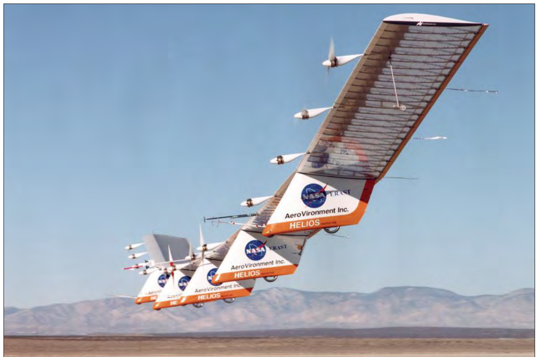
AeroVironment’s Helios prototype used battery power and solar cells. It was the precursor to Global Observer.
