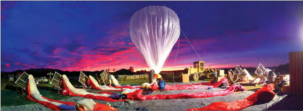
A Raven Aerostar high-altitude balloon. The craft is part of Project Loon, Google’s effort to create a network of balloons to provide wireless communications to remote populations.
