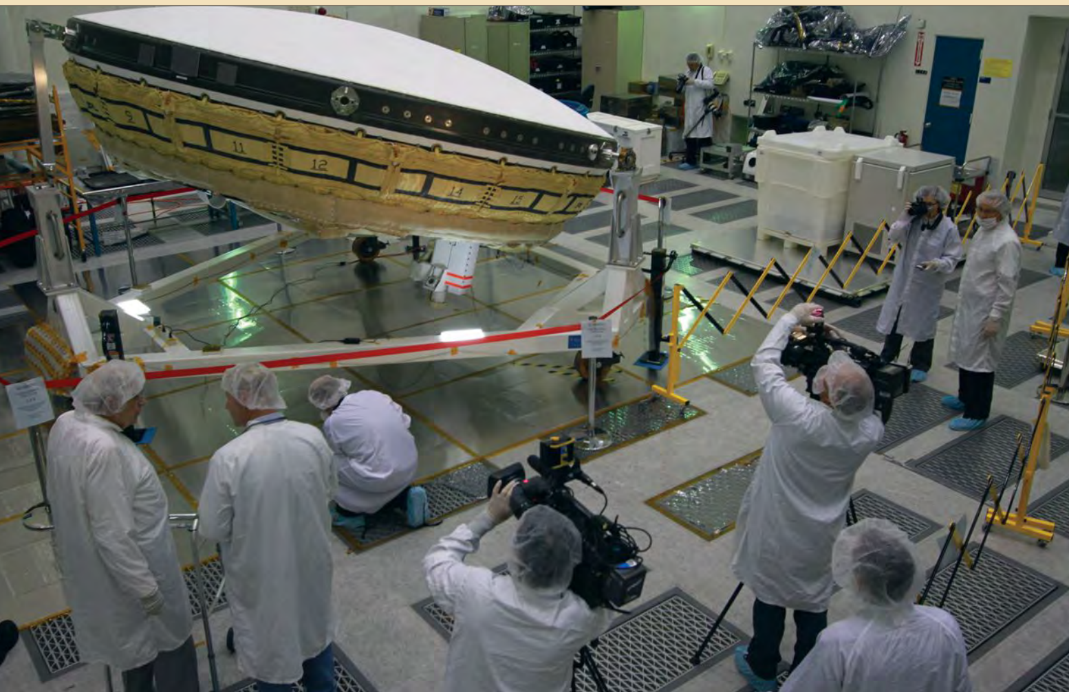
Clean room: At the Jet Propulsion Laboratory, NASA workers prepare the saucer-shaped low-density supersonic decelerator for shipment to Hawaii, where it will be launched into near-space for testing.
