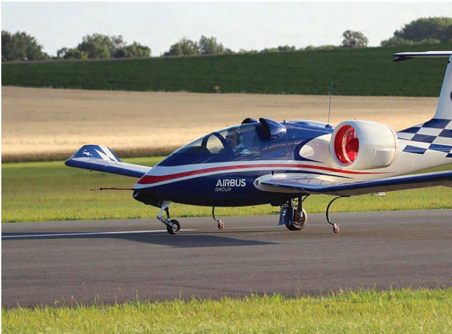
▲ Airbus' E-Fan Plus is a two-seat electric demonstrator.
