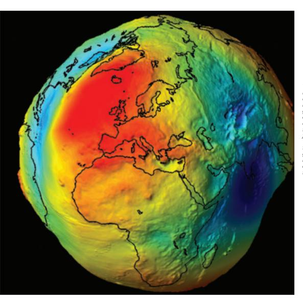
The GOCE mission is measuring high-accuracy gravity gradients and providing a global model of Earth's gravity field and of the geoid. The geoid (the surface of equal gravitational potential of a hypothetical ocean at rest) serves as the classical reference for all topographical features. The accuracy of its determination is important for surveying and geodesy, and in studies of Earth interior processes, ocean circulation, ice motion and sea-level change. Credit: ESA.
