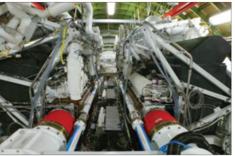
Northrop Grumman's COIL is comprised of six modules, which were installed inside a scrap 747 fuselage in the System Integration Lab at Edwards AFB. The view is looking down the center of the aisle formed by the V-6 configuration of the laser layout. USAF Photo.
