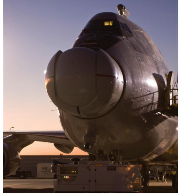
On July 21, 2009, at Edwards AFB, the Airborne Laser's first chemical flight test demonstrated the safe flow of chemicals through all laser systems.
