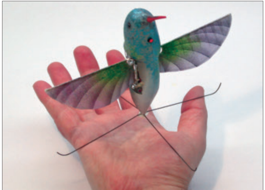
Although it did not meet DARPA's original goal of an 8-g vehicle with a 7.6-cm wingspan, the Nano is about the same size as the largest of the hummingbird species. Courtesy AeroVironment.
