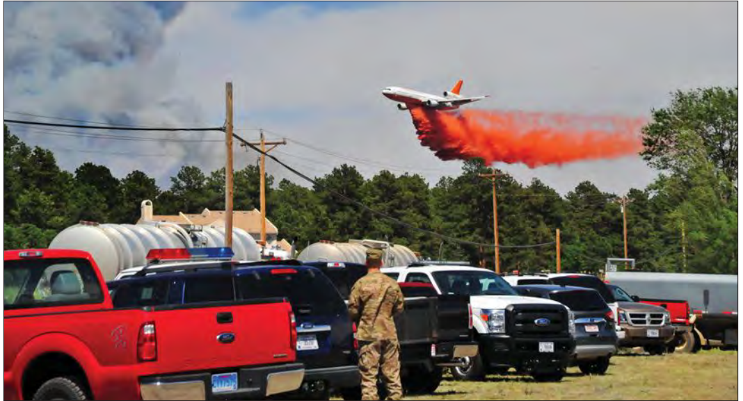
10 Tanker Air Carrier operates two converted DC-10 airliners each fitted with an 11,600-gallon retardant tank.
