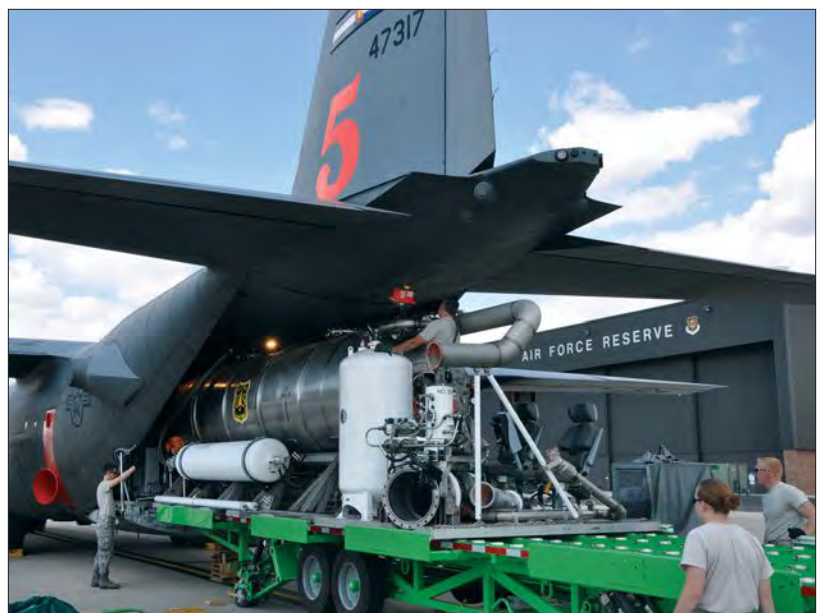
When there aren't enough commercial airtankers, the Forest Service puts its Modular Airborne Firefighting Systems into service. The portable 3,000-gallon retardant systems are rolled aboard Air Force C-130 aircraft.
