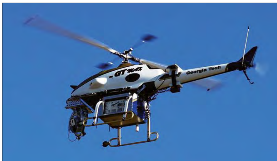
RMAX: Research on a Yamaha RMAX unmanned helicopter at Georgia Tech benefits from a new technique that provides accurate and far faster modeling of dynamic loads.
