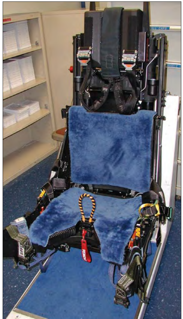
NASA has upgraded its T-38N jets with Martin Baker US16LN ejection seats to lessen danger to astronaut trainees. The seats can safely eject occupants even at zero altitude and zero airspeed.
