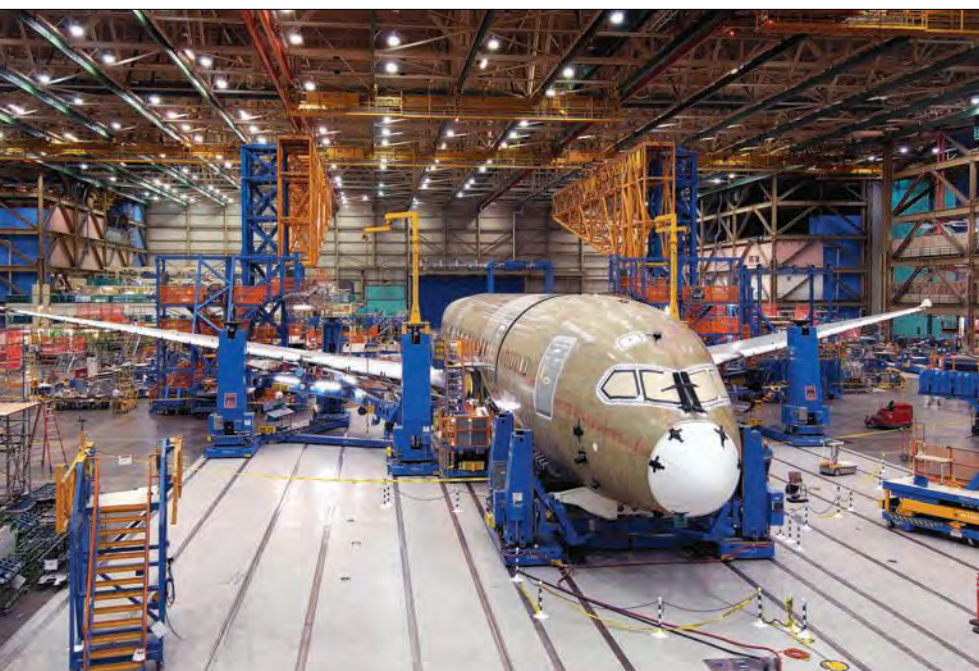
Composites make up more than half of the fuselage weight of the Boeing 787 Dreamliner.
