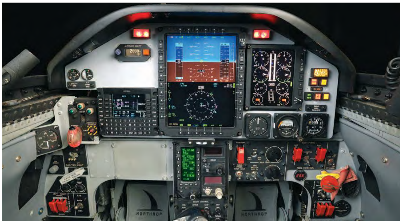
NASA's T-38N trainer jet cockpit displays don't look like that of any particular spacecraft. But its modern display technology is similar to those on the upgraded Soyuz capsules and new commercial space transports.
