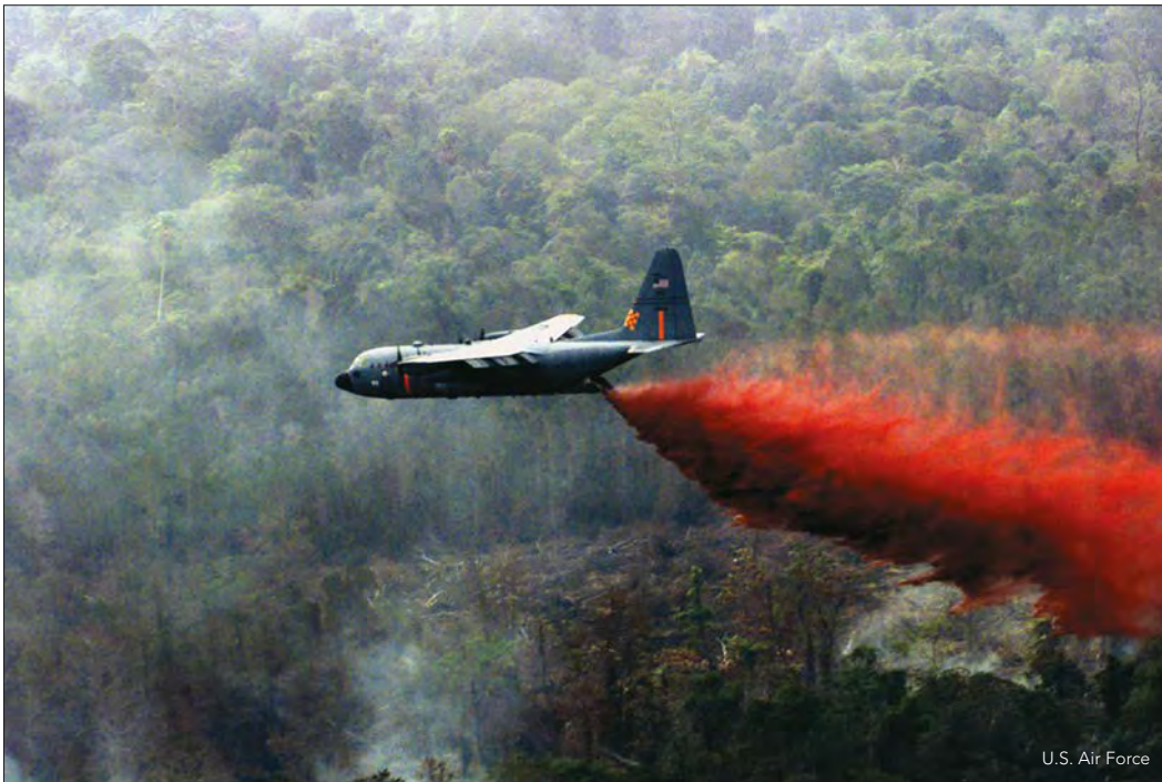
The Pentagon supplements the U.S. Forest Service's small fleet of airtankers with eight Modular Airborne Fire Fighting Systems, which are tanks of fire retardant temporarily fitted to C-130s.
