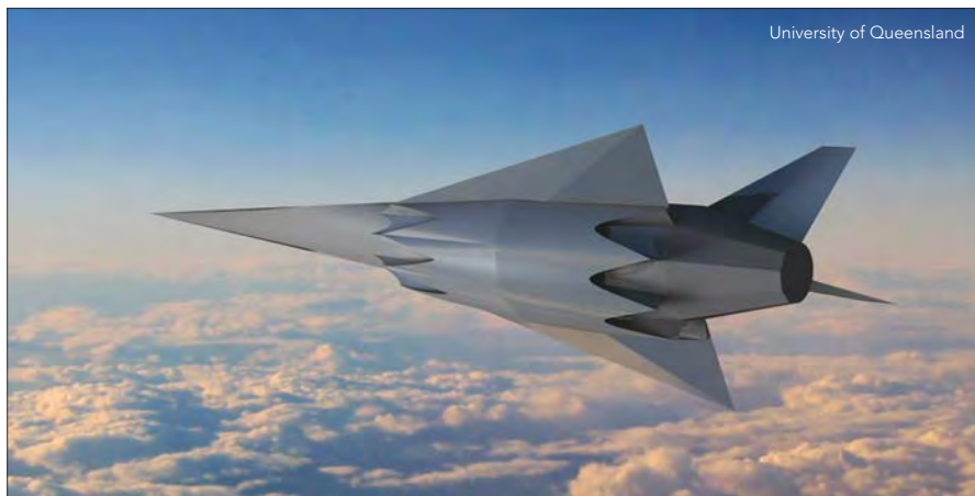
SPARTAN: To reduce launch costs, Australian engineers will need to fire up the airbreathing stage of the Scramjet Powered Accelerator for Reusable Technology Advancement at a relatively low supersonic speed, something they are still mastering.
