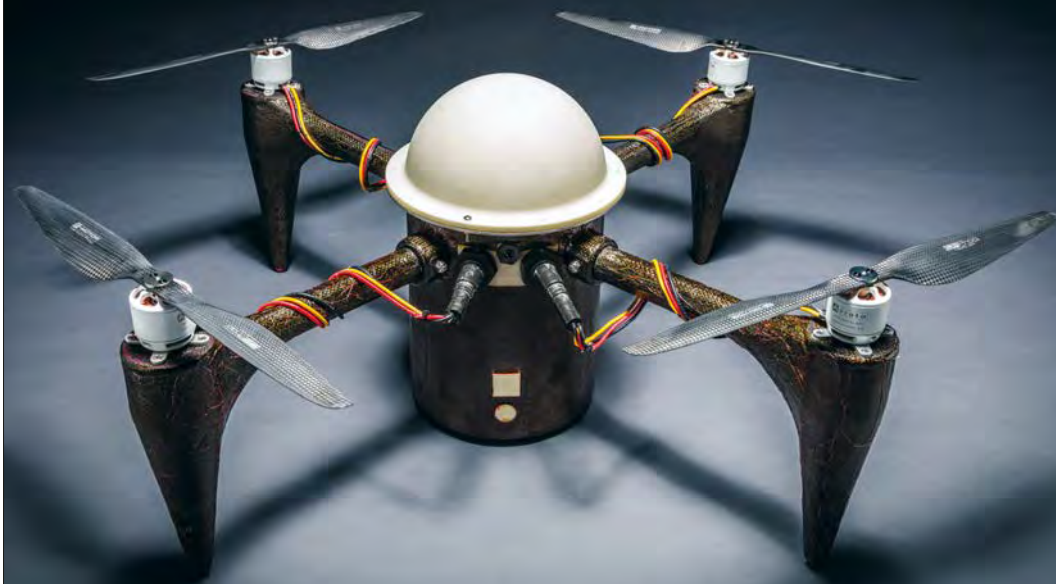
The 3D manufactured underwater drone Corrosion Resistant Aerial Covert Unmanned Nautical System is made almost entirely out of plastic, except for metal fasteners and some engine parts.
