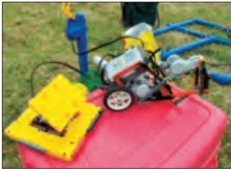
When pressed down, the team-designed LEGO® button pushes the touch sensor, which uses the NXT MINDSTORM® robot to release the catapult. (Photo courtesy of Shelley Bridenstine)
