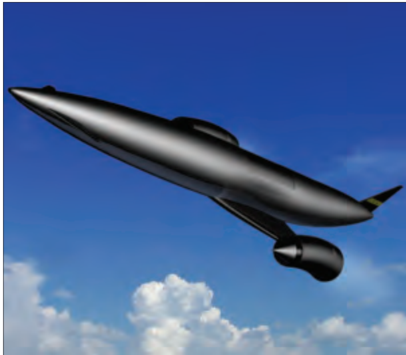
Skylon is a grandchild of the early British single-stage-to-orbit HOTOL concept. Currently being planned by Alan Bond of the U.K.'s Reaction Engines, it uses the Sabre engine, which combines turbomachinery using pre-cooled air with a hydrogen-oxygen rocket to enable flight from standstill to orbital speed.
