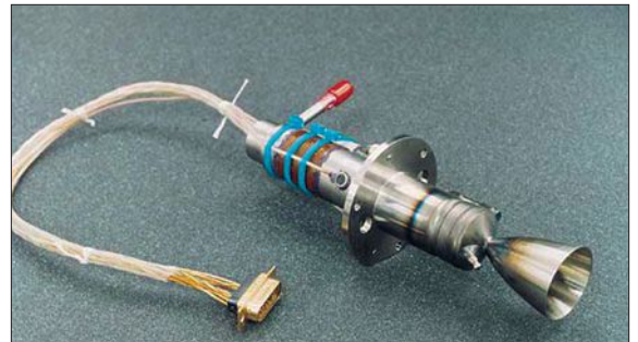
Aerojet, a member of the GPIM project, is a major manufacturer of small thrusters. This is a 22-N hydrazine thruster made by the company.
