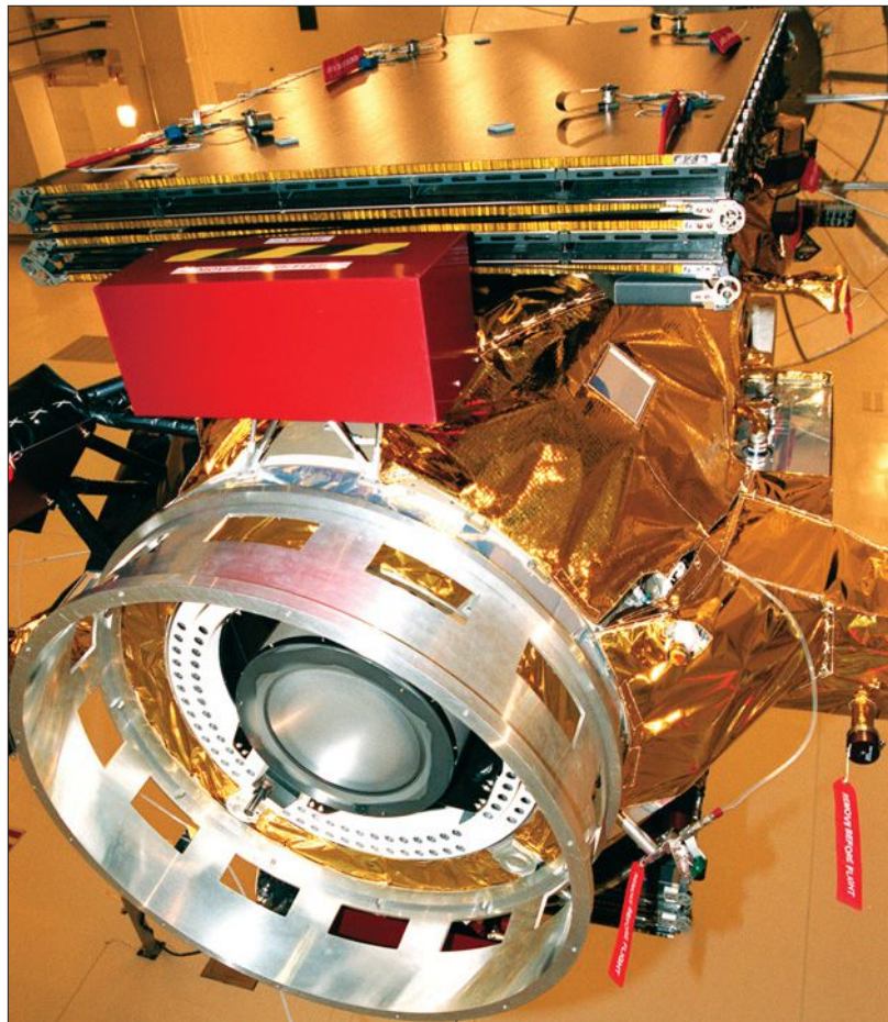
Three heritage Deep Space 1 ion propulsion engines were used to power the Dawn spacecraft.
