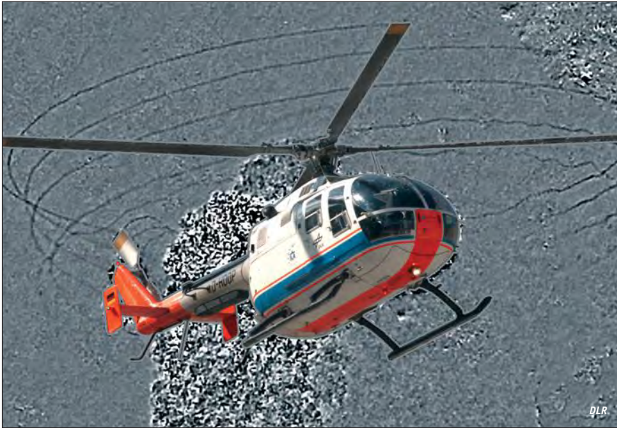
Rotor blade vortices and exhaust are visible in this Background Oriented Schlieren image, a technique pioneered by German researchers.
