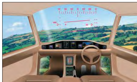
The myCopter would have car-like controls, including a steering wheel and foot pedals to increase or decrease speed.
