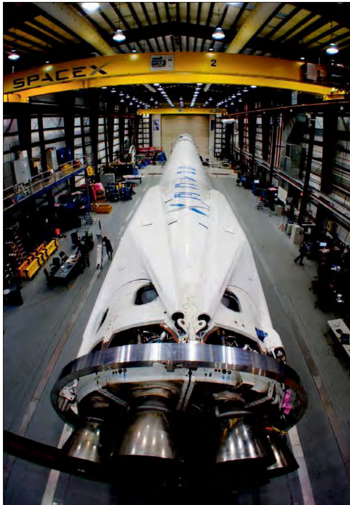
The SpaceX Falcon 9 rocket is powered by nine of the company's Merlin 1D engines, each producing 147,000 pounds of thrust at liftoff. The Falcon 9 could be certified to compete with the Atlas 5 for national security launches this year, the Air Force said.
