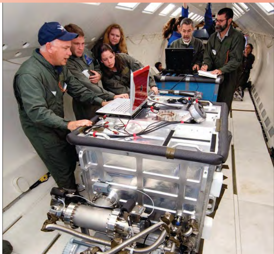
NASA researchers test an Electrodynamic Dust Shield in a vacuum chamber during reduced-gravity flights on a NASA aircraft.
