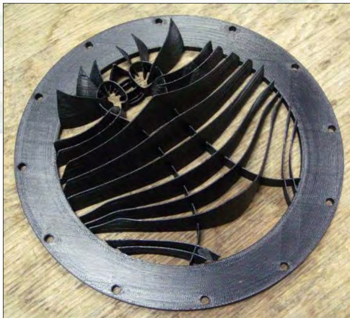
A StreamVane replicates airflow distortions of specific inlet designs in a wind tunnel. This one was made with a 3-D printer.
