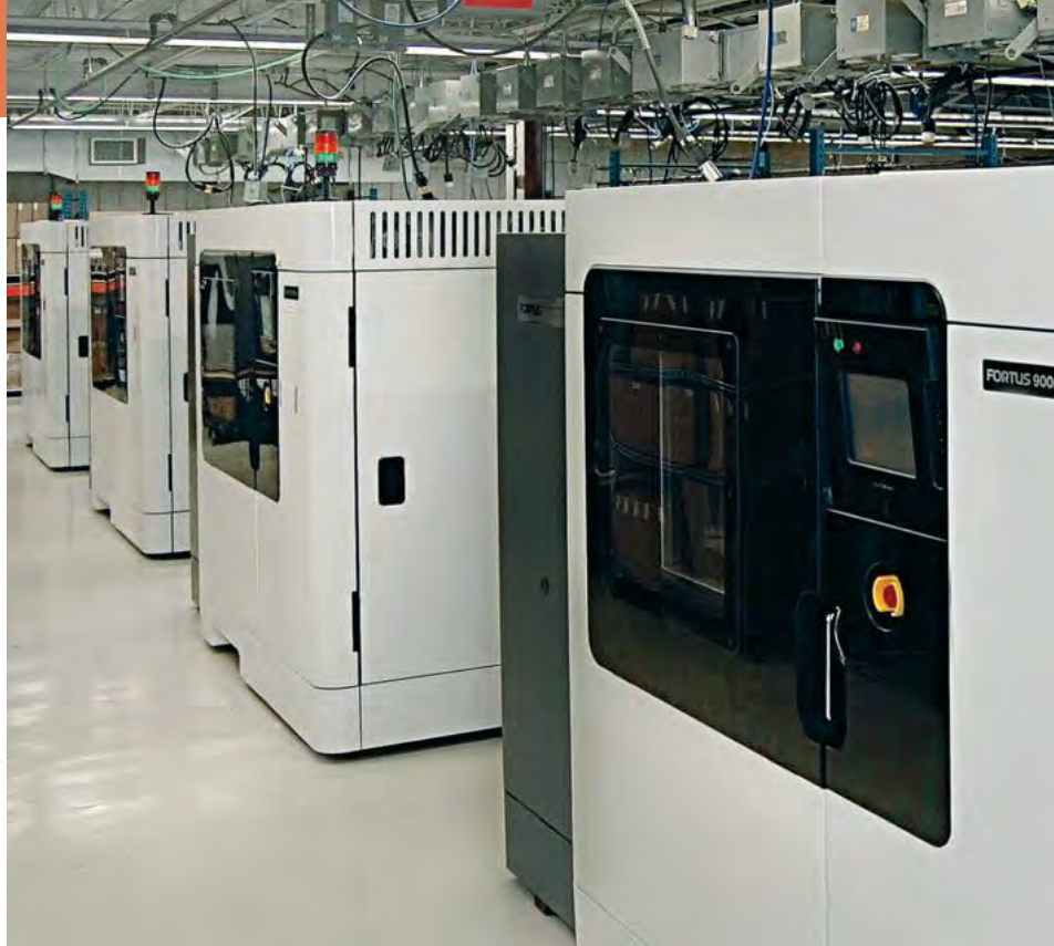
Stratasys’ 3-D printers can produce objects in a variety of materials, including ULTEM 9085, a thermoplastic the company uses to print antenna supports for Formosat-7 satellites.
