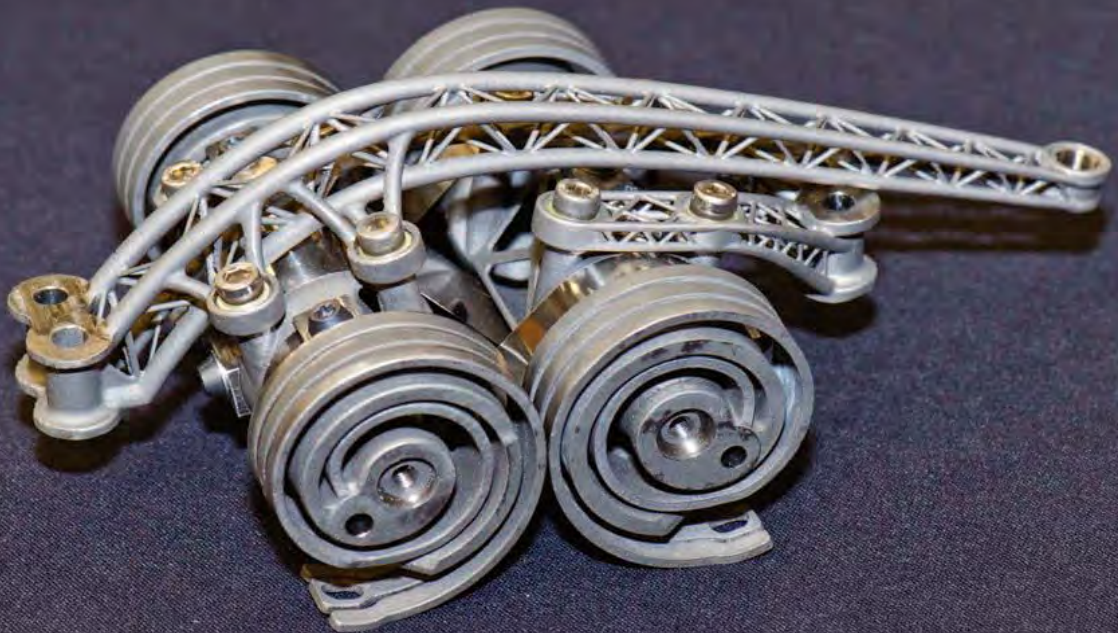
Thales Alenia Space used a 3-D printer to produce a prototype deployment mechanism for satellite solar panels. The titanium device has fewer parts and about one-fifth the mass of a similar, conventionally produced mechanism, according to the European Space Agency.
