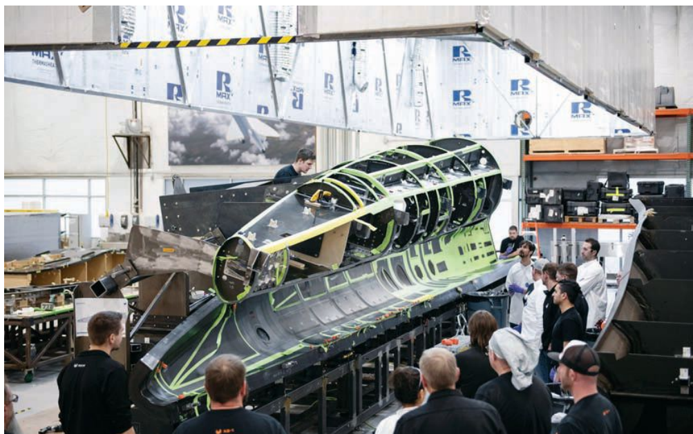
► The XB-1 cockpit is bonded in Boom’s hangar in Colorado.
