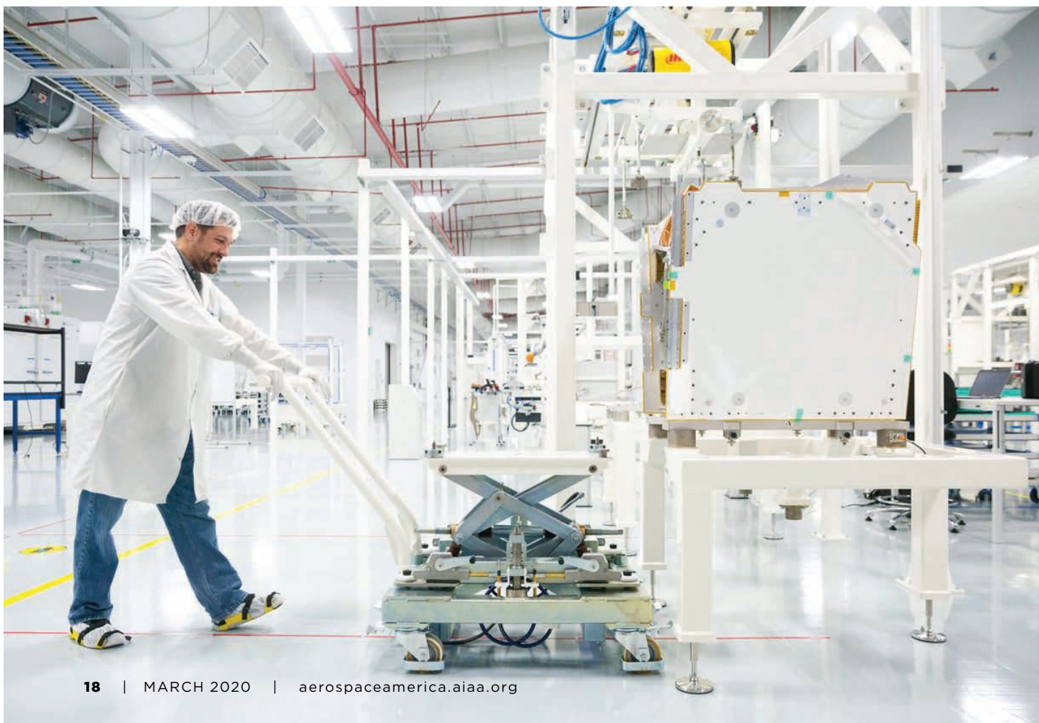
▼ An engineer prepares to move a completed OneWeb satellite to a chamber to test for extreme temperatures. OneWeb Satellites
