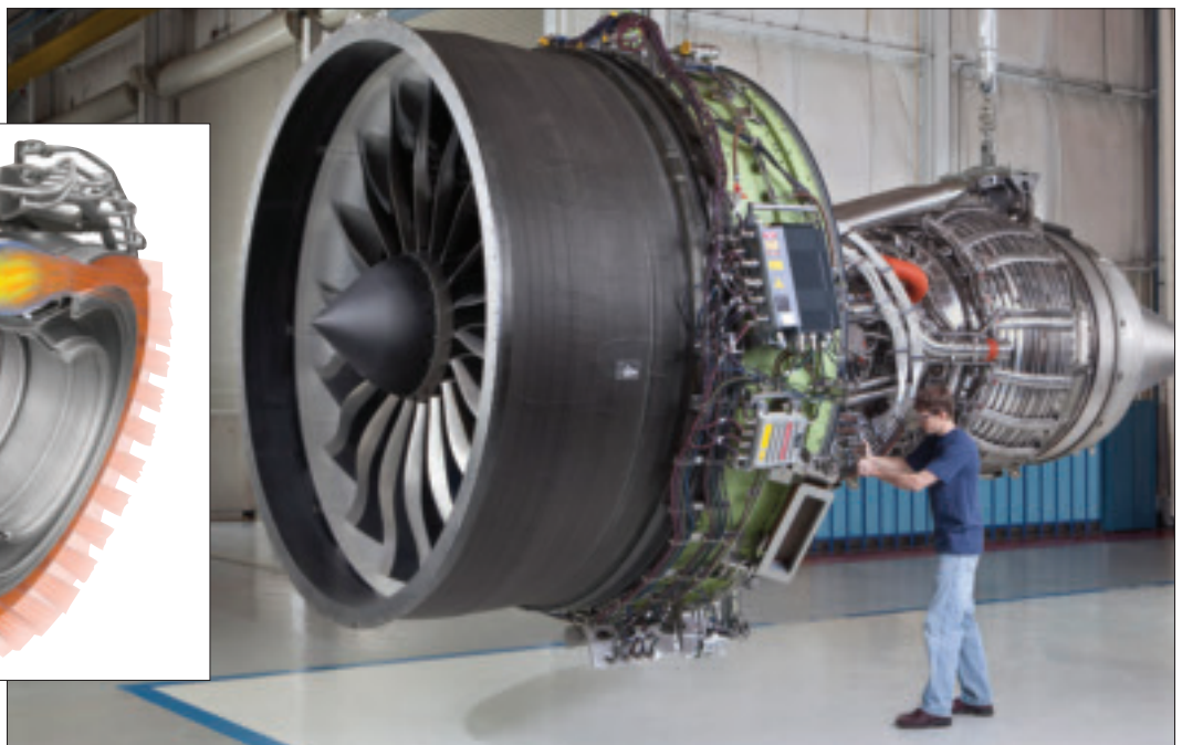
General Electric’s GEnx-1B engine includes the company’s TAPS combustor technology to reduce emissions. Credit: General Electric.
