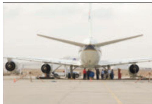
Test instrumentation is set up behind the inboard engines of NASA’s DC-8 airborne science laboratory during alternative fuels emissions and performance testing. Image credit: NASA Dryden/Tom Tschida.
