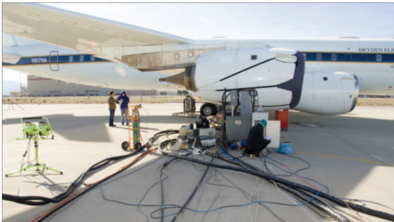
A maze of wires and tubing that connects data-collection instrumentation to the control centers is laid out on the pavement beside the DC-8 flying laboratory during synthetic fuels emission and performance testing.
