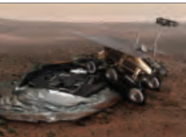
The ExoMars descent lander (above) would deliver the rover (below) to a specific location using an inflatable braking device or parachute system. Using conventional solar arrays to generate electricity, the rover will be able to travel a few kilometers over the rocky orange-red surface of Mars.
