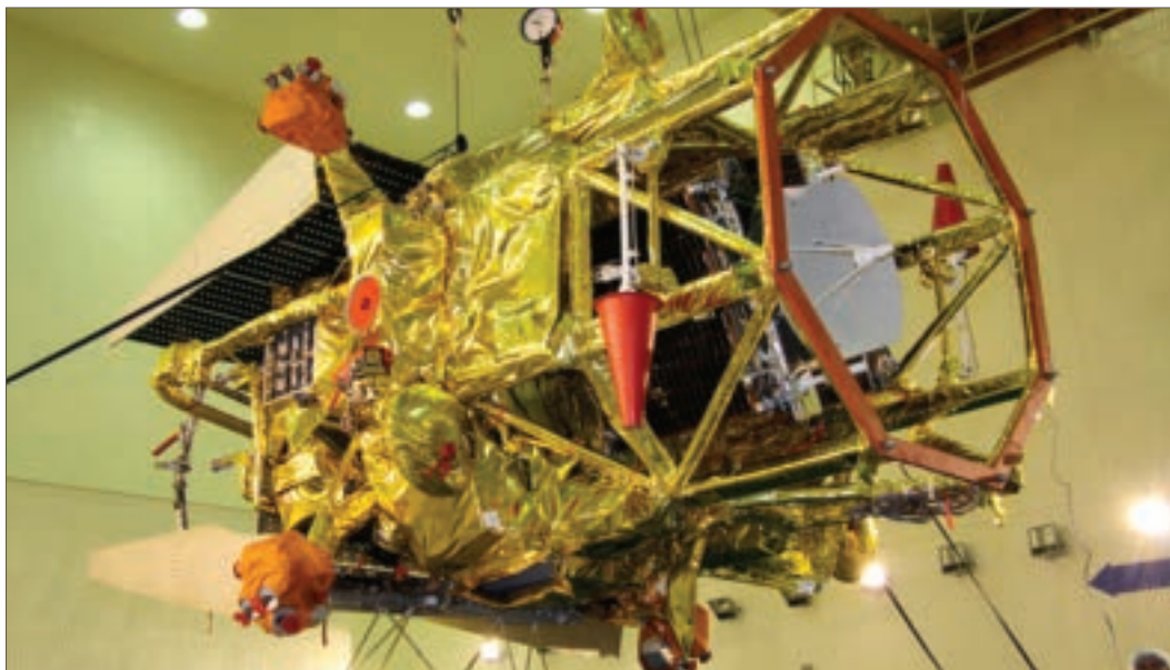
The failed Phobos-Grunt spacecraft did not perform its scheduled burn to begin a trajectory to Mars, later tumbling to Earth in an uncontrolled reentry. Courtesy: National Space Science Data Center.
