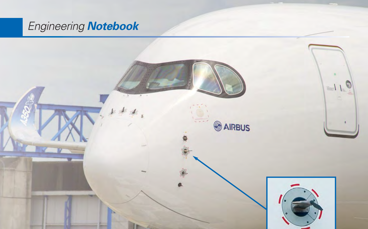
Closer look: Mounted on an Airbus A350, the Pitot tube (blue arrow) is used by planes to measure airspeed. Inset shows a Pitot tube – the pencil-point shape – with a static port and black angle-of-attack vane.
