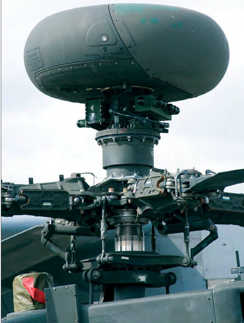
Above the rotor blades is the donut-shaped radome. It houses either data-link hardware or the fire-control radar that spots targets.
