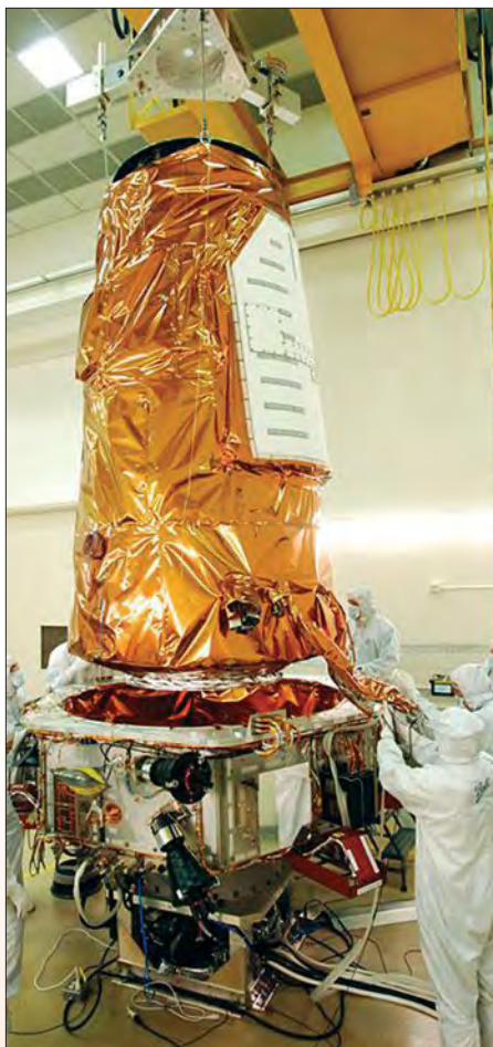
Lowering the Kepler space telescope photometer onto the satellite. Lepore advocates for this and other Ball Aerospace programs at the company's Washington, D.C., office.
