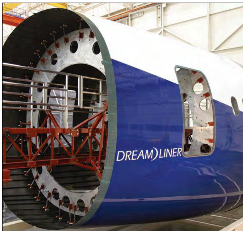
The use of composites in the 787 Dreamliner reduces the number of components and improves aerodynamic performance.
