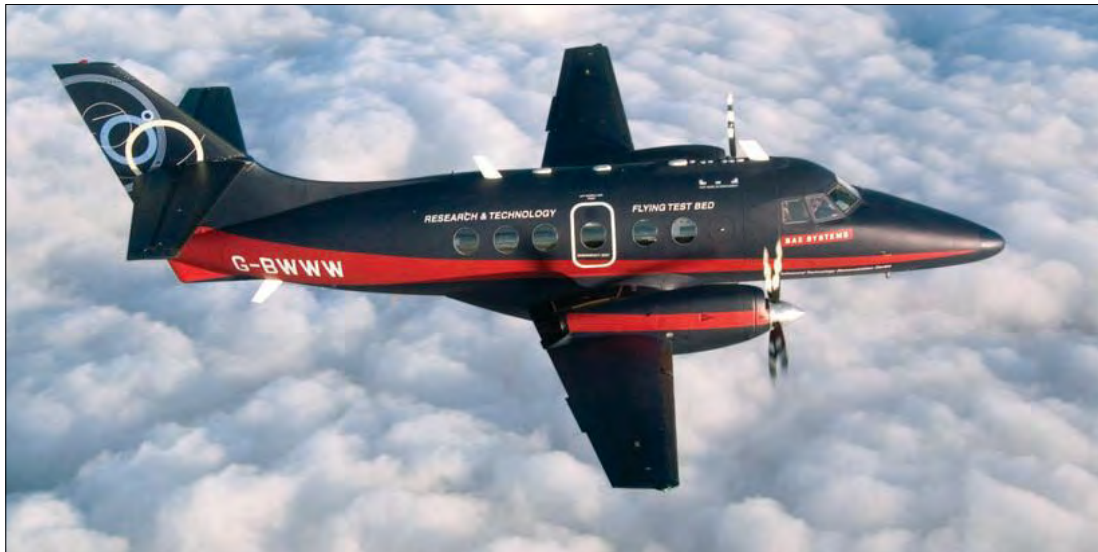
In 2013, a BAE Systems Jetstream was flown over the U.K. by a pilot on the ground, with backup pilots aboard the plane.
