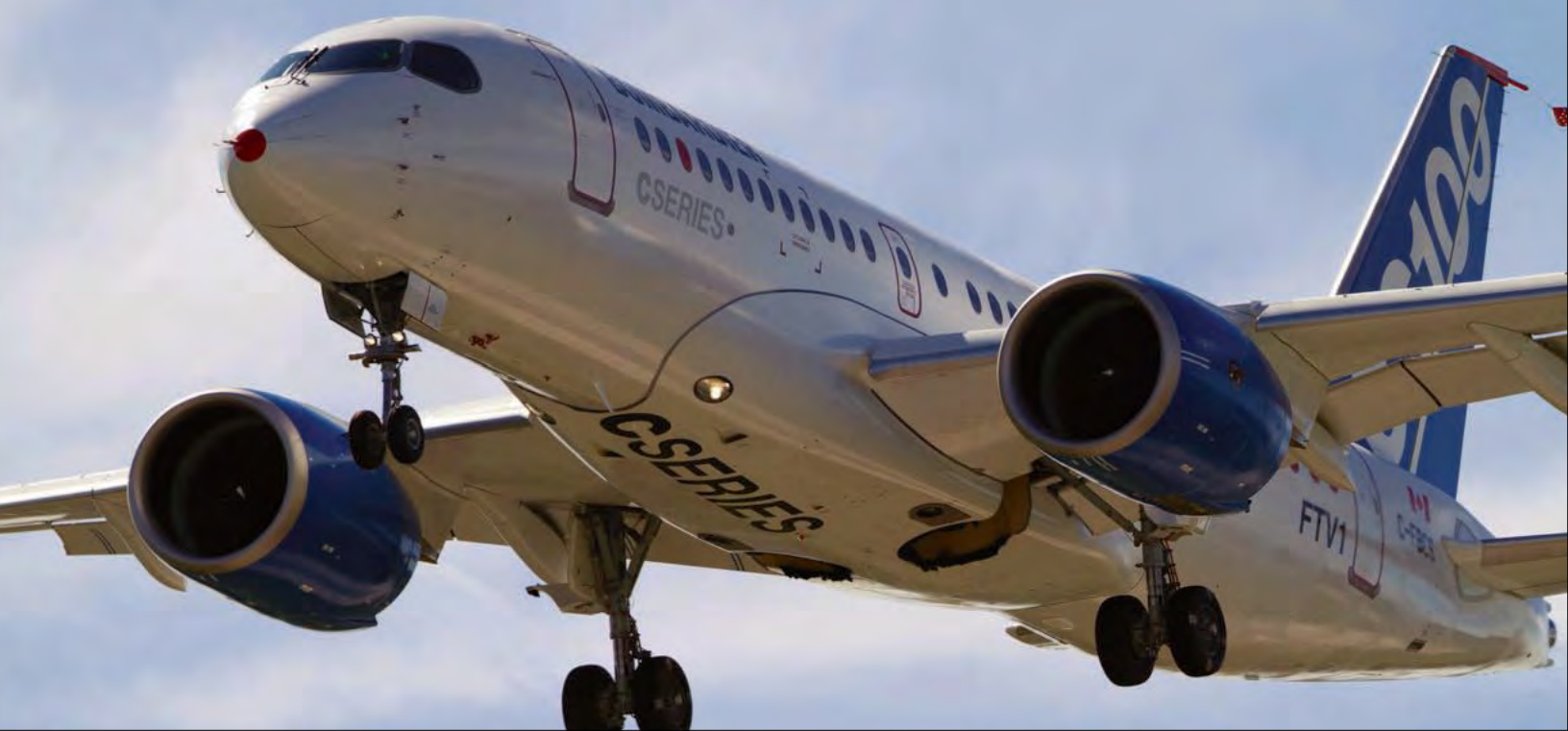
Bombardier's C Series regional jets use composites for the rear fuselage, tail sections, wings and engine nacelles, shaving 2,000 pounds.
