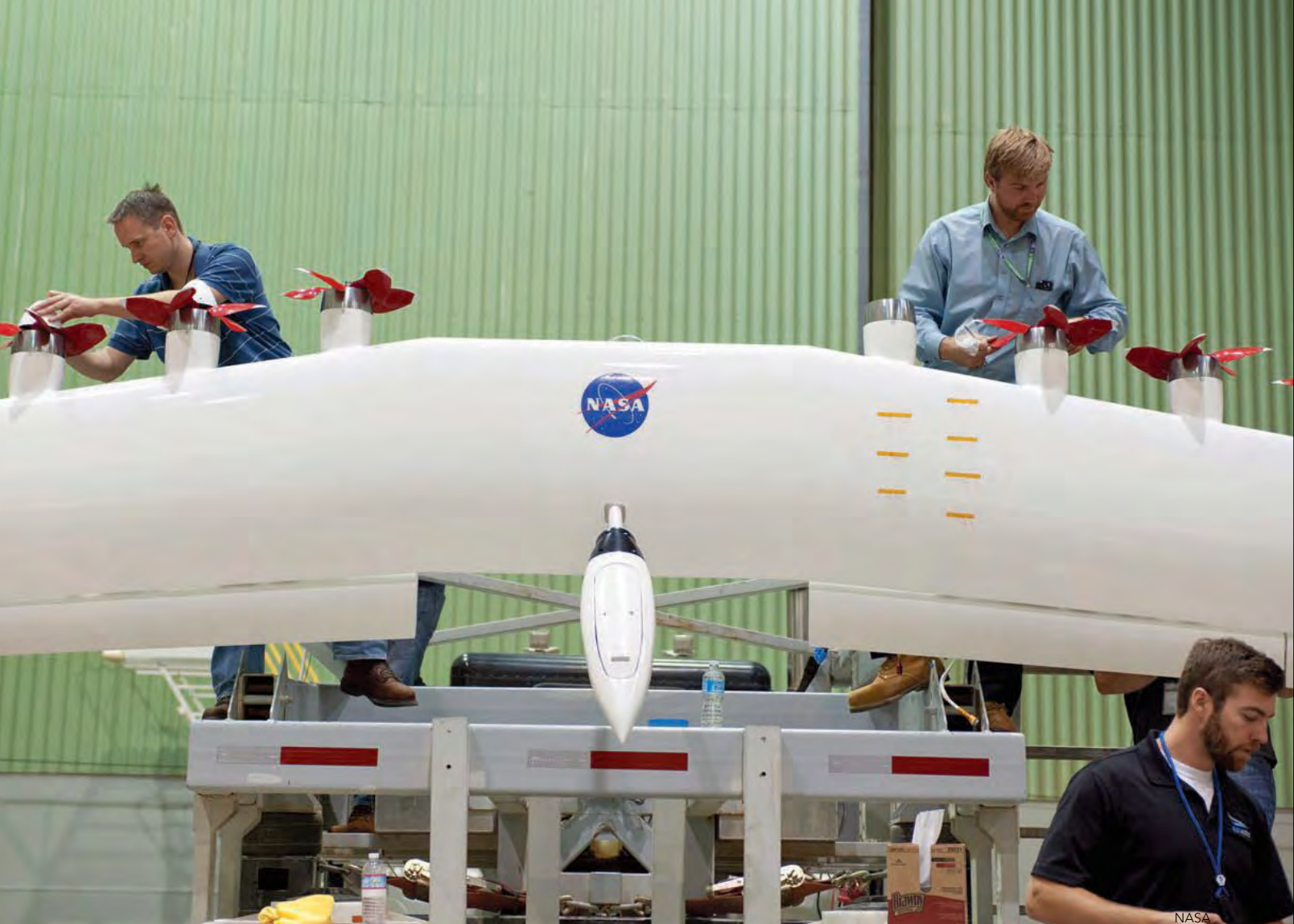
Engineers at NASA's Armstrong Flight Research Center modify the wing of an experimental plane called SCEPTOR, Scalable Convergent Electric Propulsion Technology and Operations Research. NASA is also replacing the aircraft's two fuel tanks with lithium-ion batteries.
