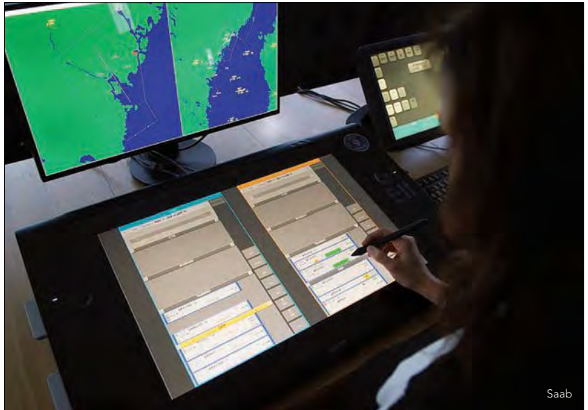
A remote air traffic controller in Sundsvall, Sweden, guides an airplane to a landing at the Örnsköldsvik airport about 140 kilometers away. In 2015, Örnsköldsvik became the world's first airport to use the Saab remote tower technology.
