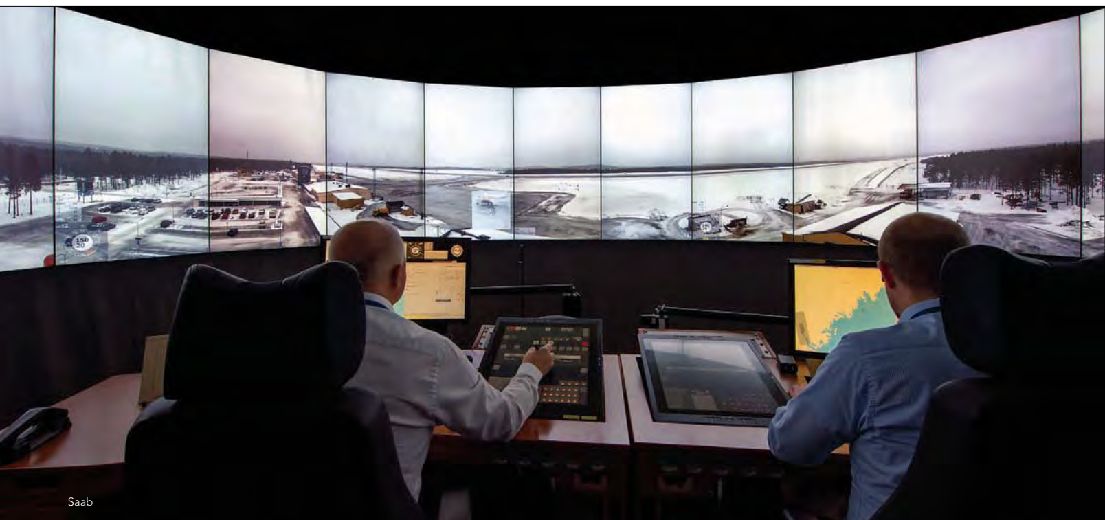
Saab Sensis is expanding its Remote Air Control Tower technology from Europe into the U.S. The technology enables off-site controllers to direct flights into non-towered airports, which otherwise require pilots to follow specific operating rules to take off and land.
