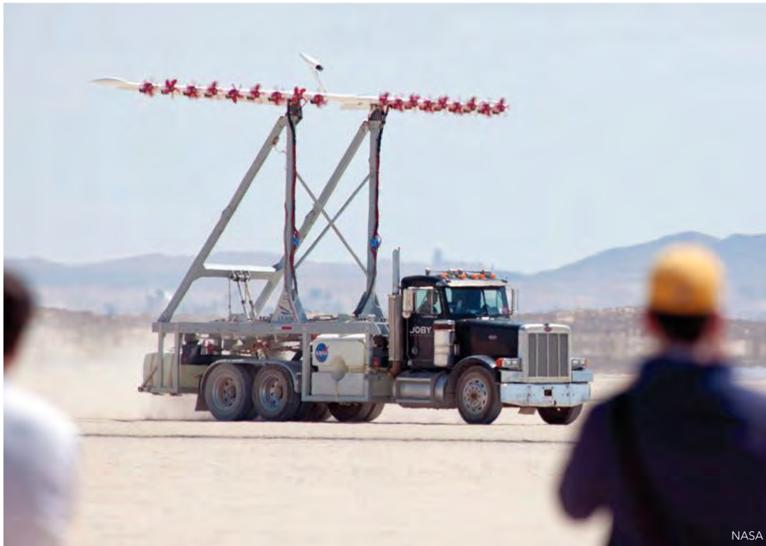
NASA is testing an experimental wing with electrically driven propellers as part of its Leading Edge Asynchronous Propeller Technology program.
