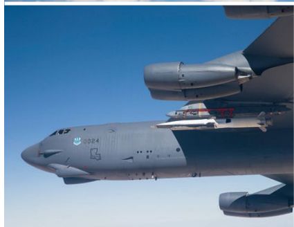
The U.S. Air Force's X-51A Waverider previously held the record for longest air-breathing hypersonic flight. Once released from the wing of a B-52 Stratofortress, the demonstrator's scramjet engine lit and accelerated the aircraft for 210 seconds during the final test flight of the program in May 2013.
