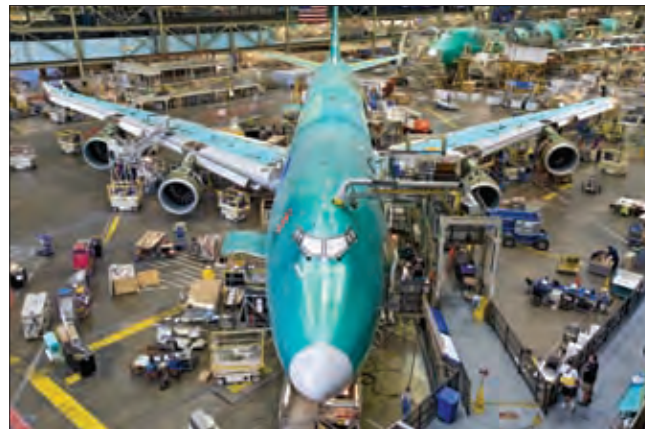
A milestone was reached in the assembly of the Boeing 747-8 freighter as mechanics completed installation of GENx-2B engines on Airplane 1.
