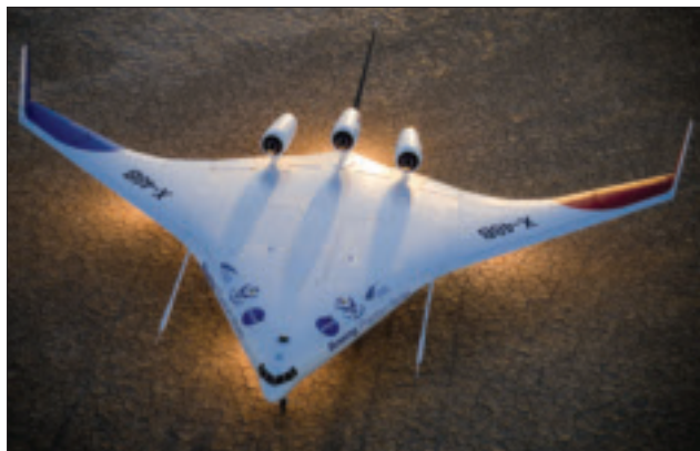
The X-48 blended wing body design promises lower fuel costs, which will continue to receive high priority.
