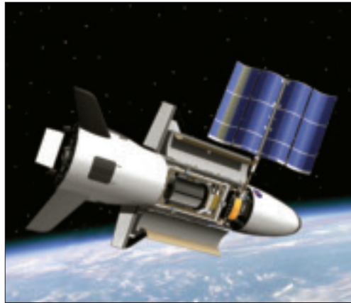
In this NASA graphic, the X-37B flies in space with its payload bay open and solar array extended. NASA graphic.
