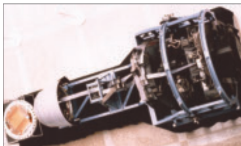
Corona cameras improved over the years, providing progressively sharper imagery, with ground resolution of objects reduced to less than 5 ft.
