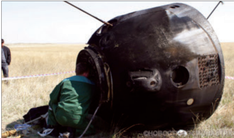
Heat damage is evident on the Soyuz TMA-11 descent module after landing on April 19, 2008. Astronauts will have to respond to similar in-flight emergencies in the era of ISS, Soyuz, and commercial crew spacecraft. (Photo: Novosti/Aleksandr Pantyukhin)
